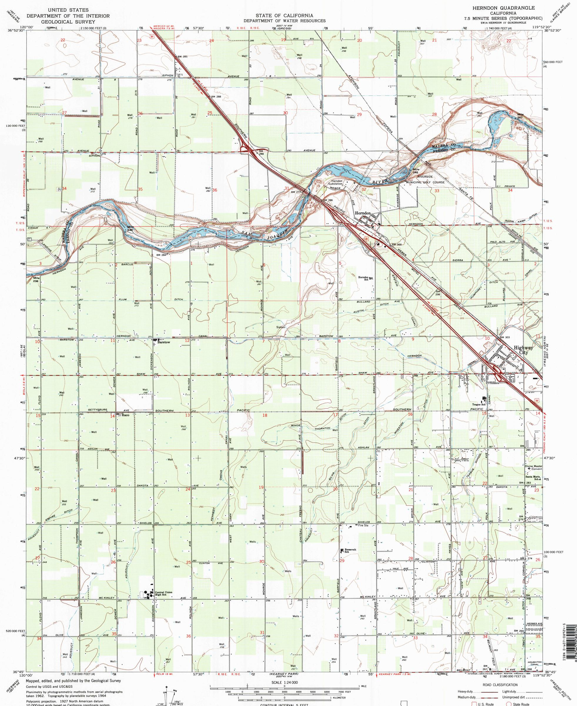
Polyconic projection. 1927 North American datum 10,000-foot grids based on California coordinate system, zones 4 and 3 1000-meter Universal Transverse Mercator grid ticks, zone 11, shown in blue
