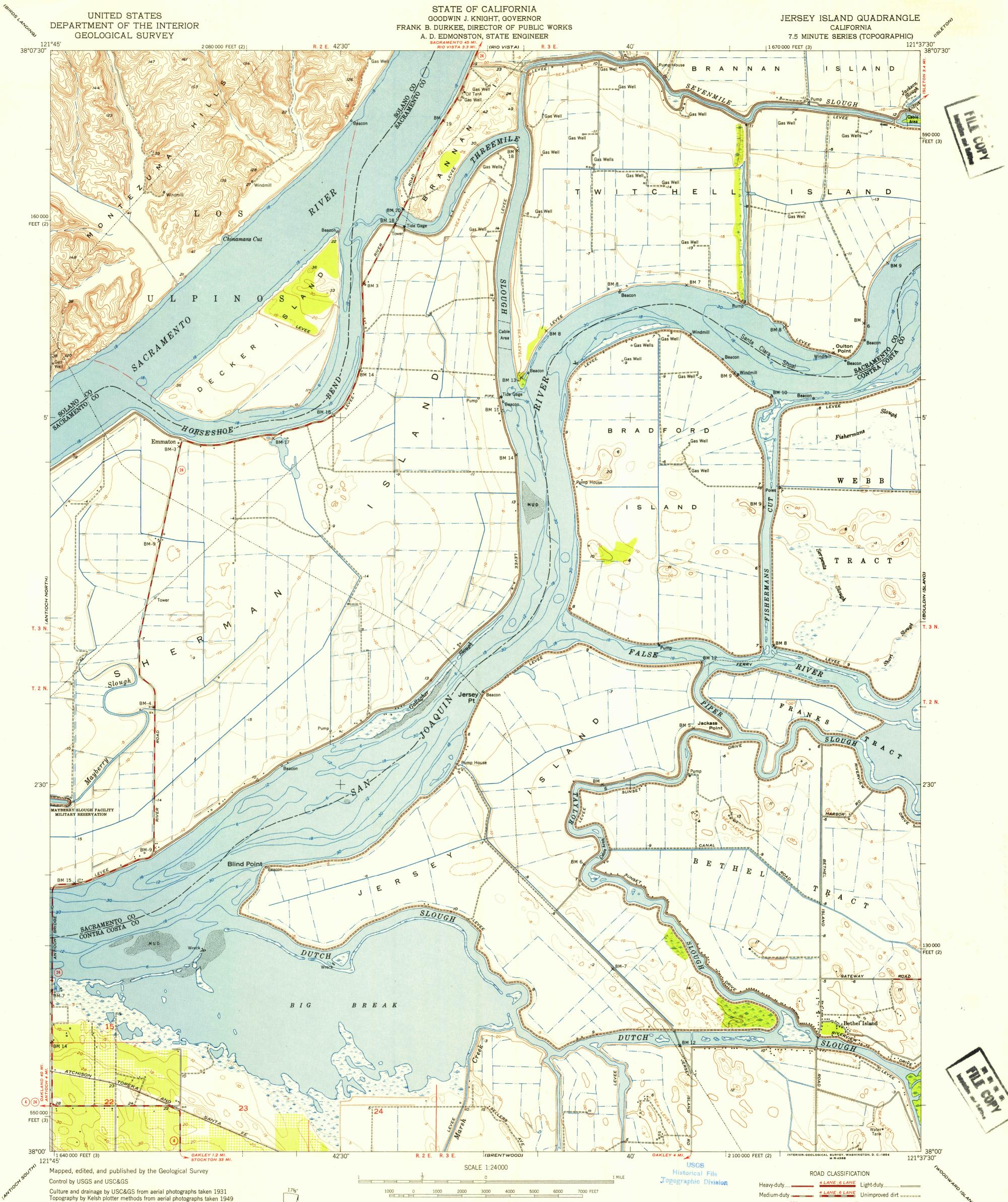
and by plane-table surveys 1952 Hydrography compiled from USC&GS Chart 5527 Polyconic projection. 1927 North American datum 10,000-foot grids based on California coordinate system, zones 2 and 3 Los Ulpinos land grant boundary not shown where APPROXIMATE MEAN DECLINATION, 1952 coincident with river bank The position of township and range numbers in unsectionized areas are approximate
