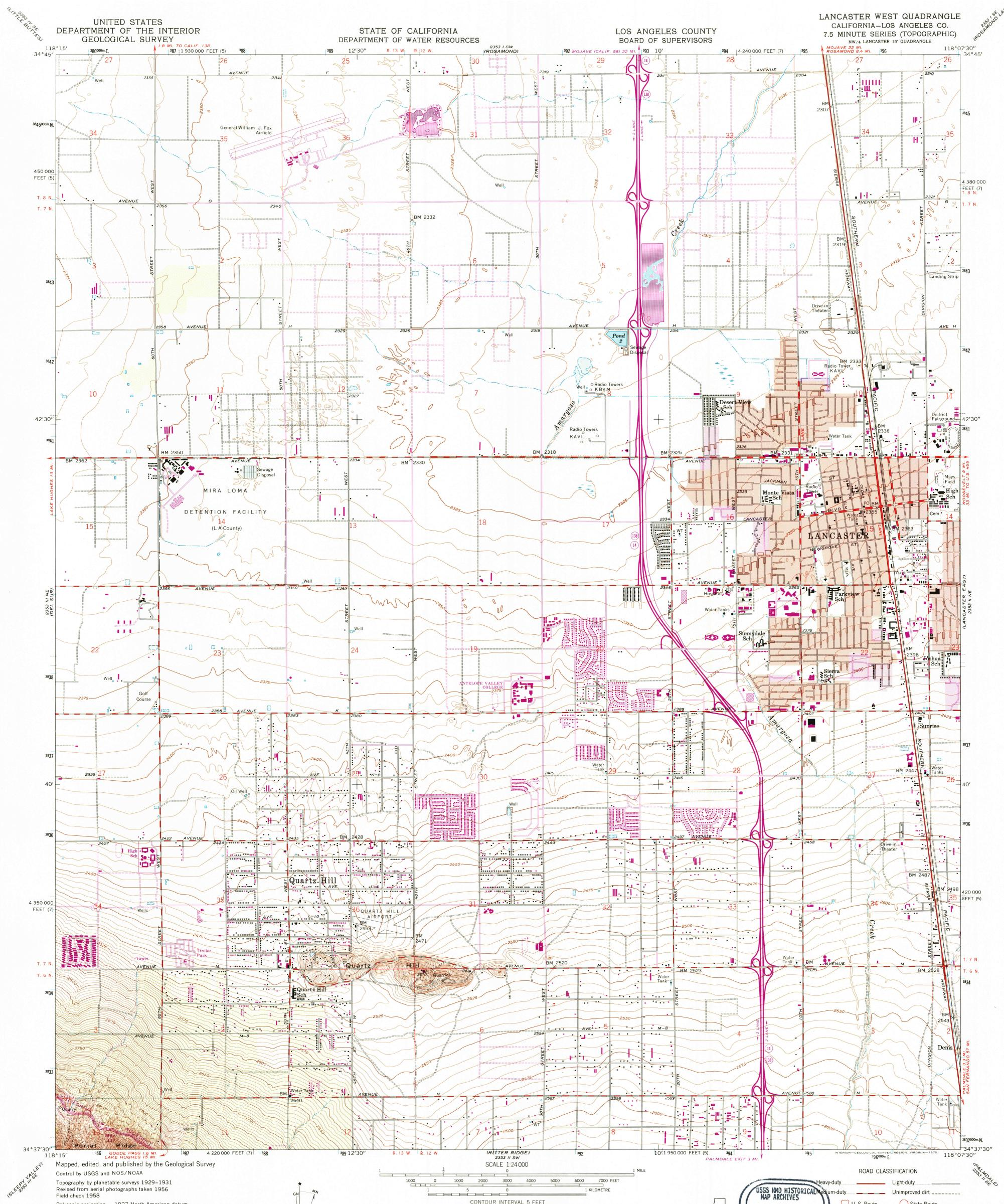
Polyconic projection: 1927 North American datum 10,000-foot grids based on California coordinate system, zones 5 and 7 1000-metre Universal Transverse Mercator grid ticks, zone 11, shown in blue
