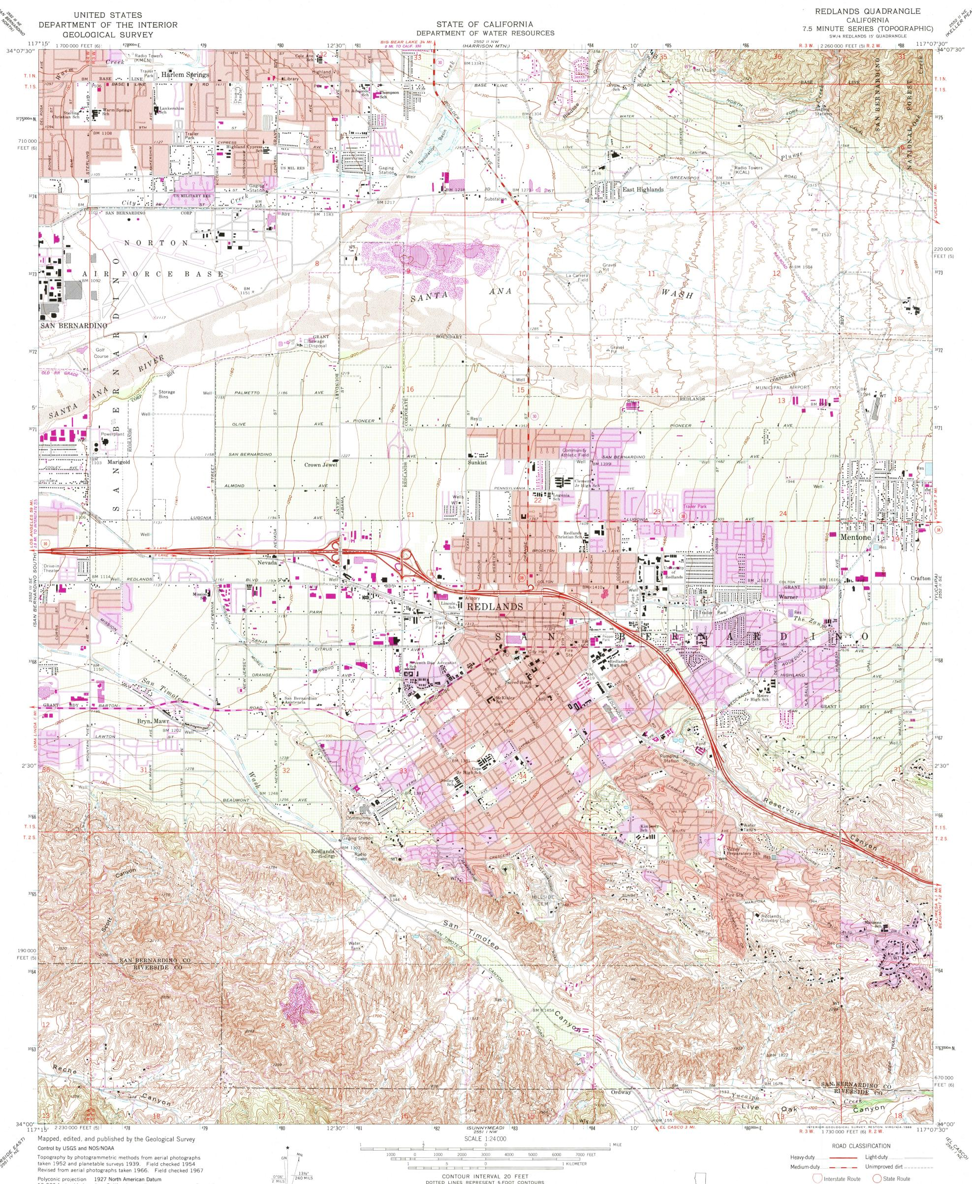
Polyconic projection 1927 North American Datum 10,000-foot grids based on California coordinate system, zones 5 and 6 1000-meter Universal Transverse Mercator grid ticks, zone 11, shown in blue To place on the predicted North American Datum 1983 move the projection lines 1 meter north and 82 meters east as shown by dashed corner ticks
