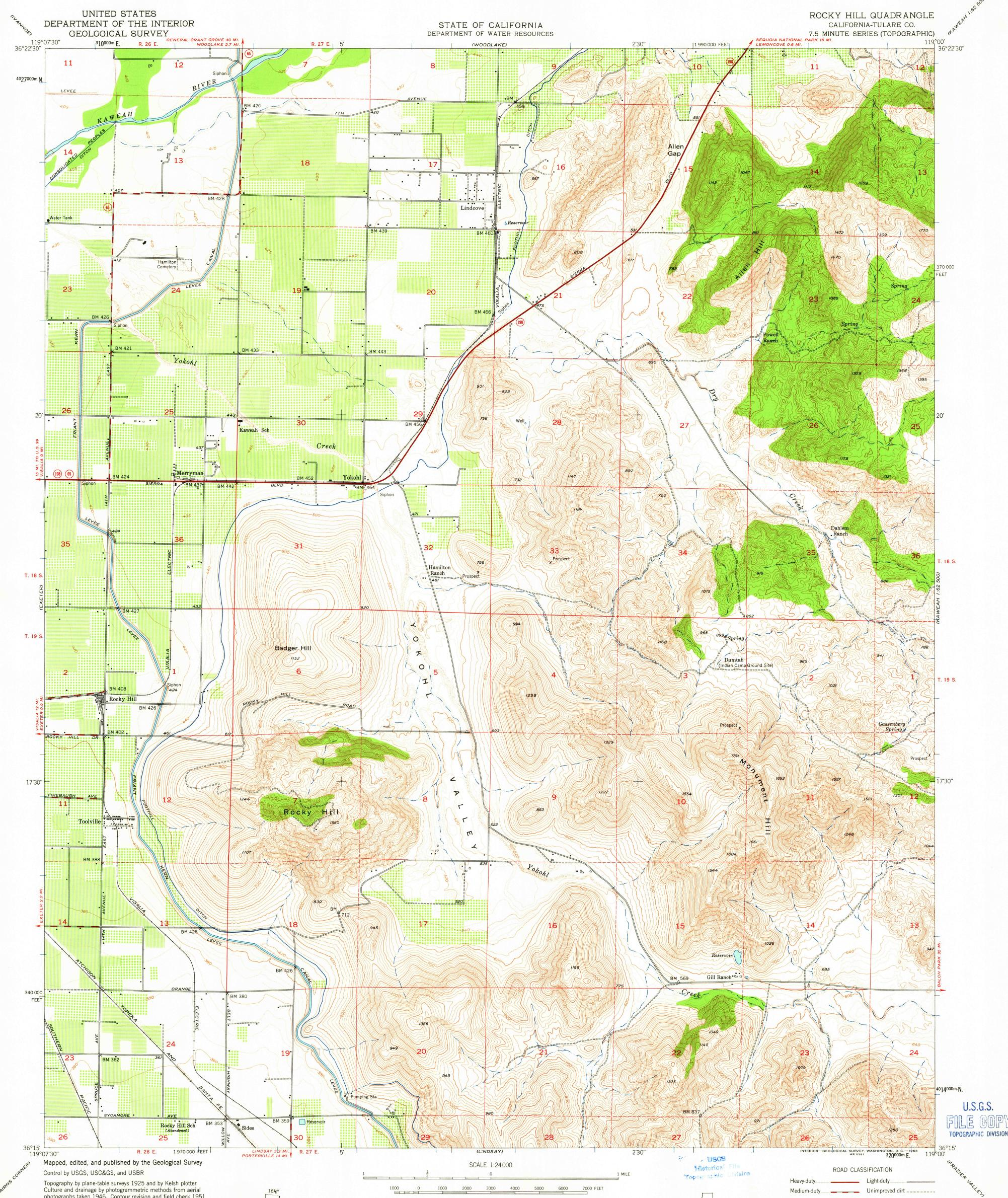
Culture and drainage by photogrammetric methods from aerial photographs taken 1946. Contour revision and field check 1951 Polyconic projection. 1927 North American datum NORTH 10,000-foot grid based on California coordinate system, zone 4 Dashed land lines indicate approximate locations RUE Dotted land lines were established by private survey Unchecked elevations are shown in brown APPROXIMATE MEAN 1000-meter Universal Transverse Mercator grid ticks, DECLINATION, 1951 zone 11, shown in blue
