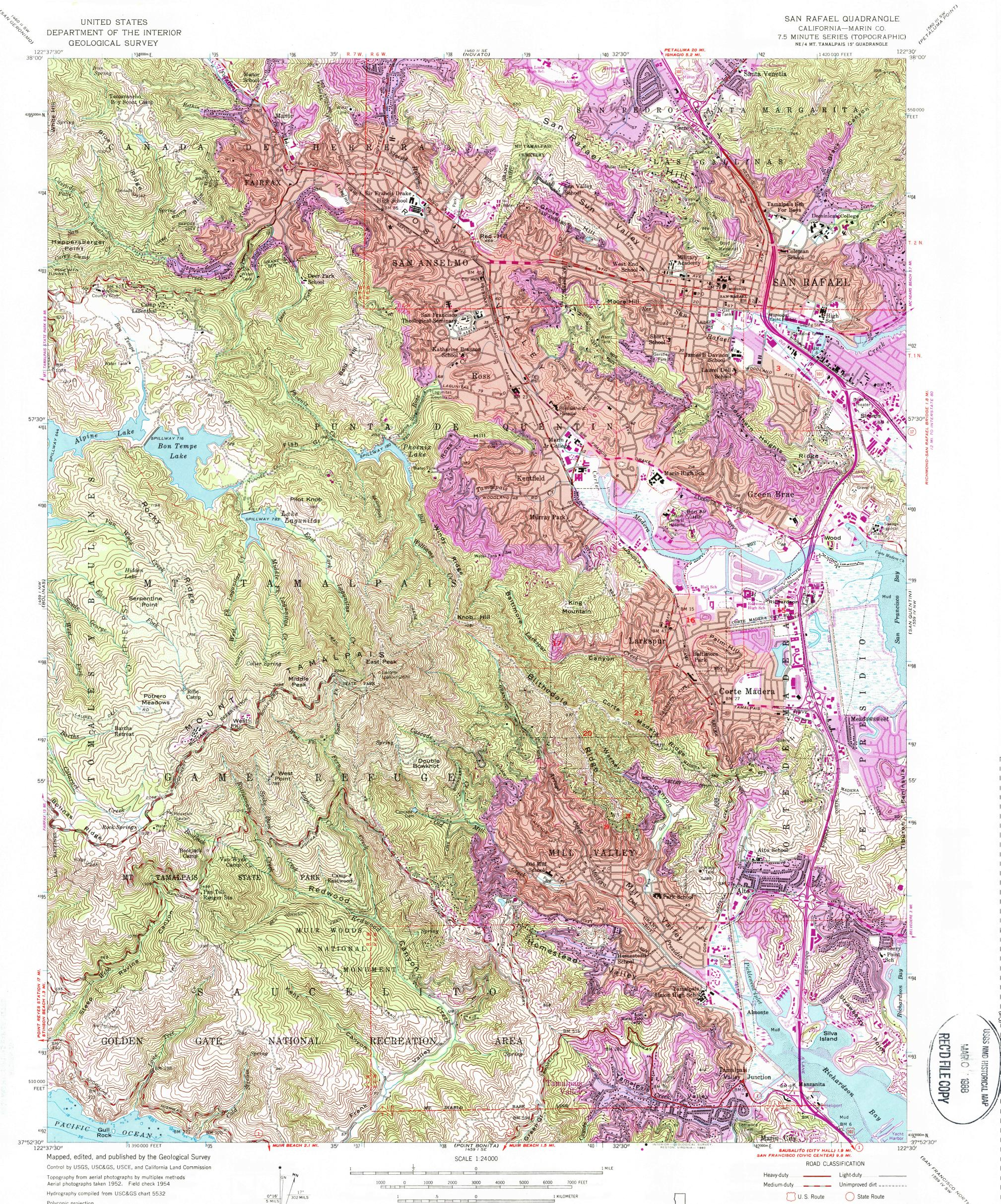
Polyconic projection 10,000-foot grid based on California coordinate system, zone 3 1000-meter Universal Transverse Mercator grid ticks, zone 10, shown in blue. 1927 North American Datum To place on the predicted North American Datum 1983 move the projection lines 15 meters north and 96 meters east as shown by dashed corner ticks
