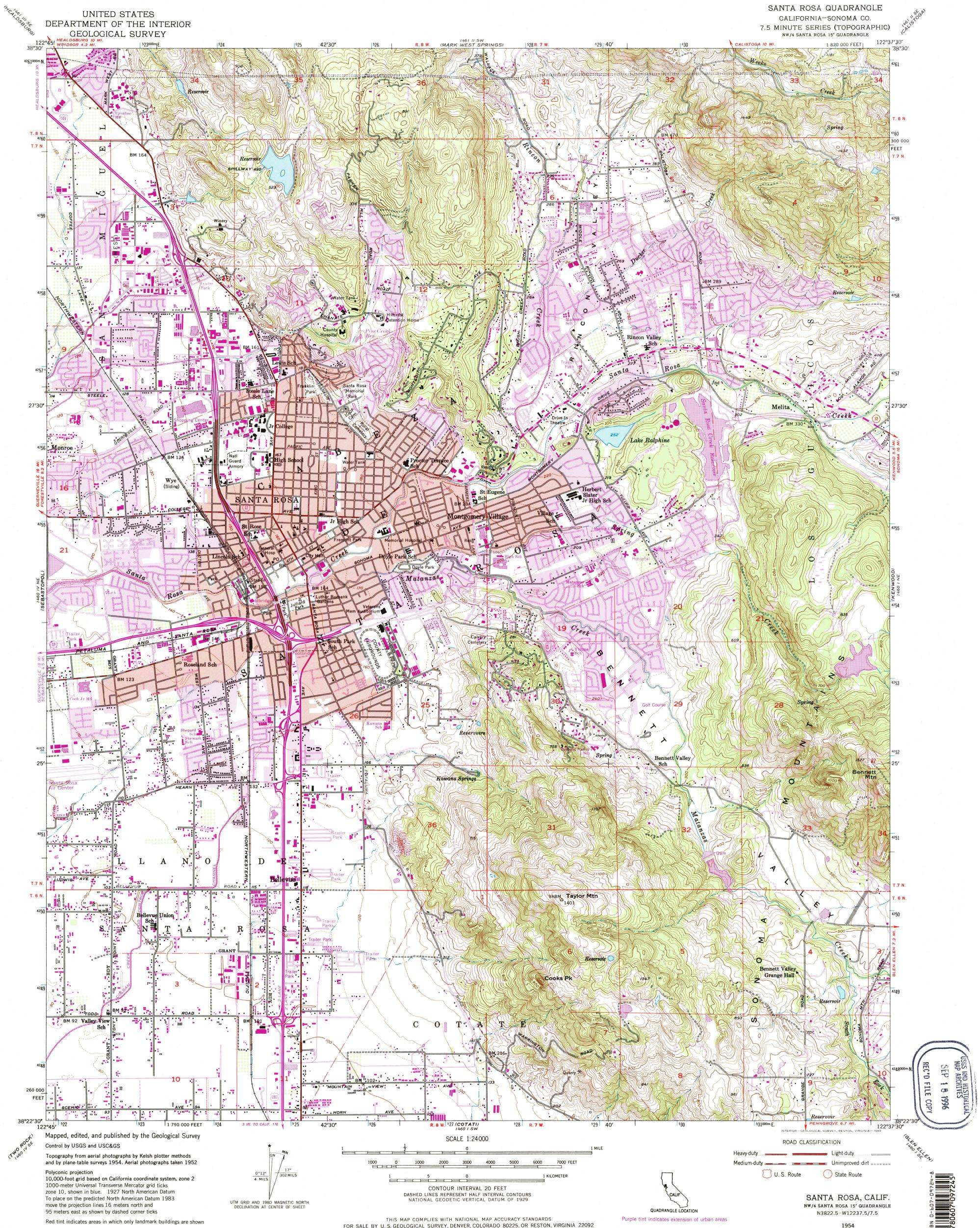
10,000-foot grid based on California coordinate system, zone 2 1000-meter Universal Transverse Mercator grid ticks zone 10, shown in blue. 1927 North American Datum To place on the predicted North American Datum 1983 move the projection lines 16 meters north and 95 meters east as shown by dashed corner ticks
