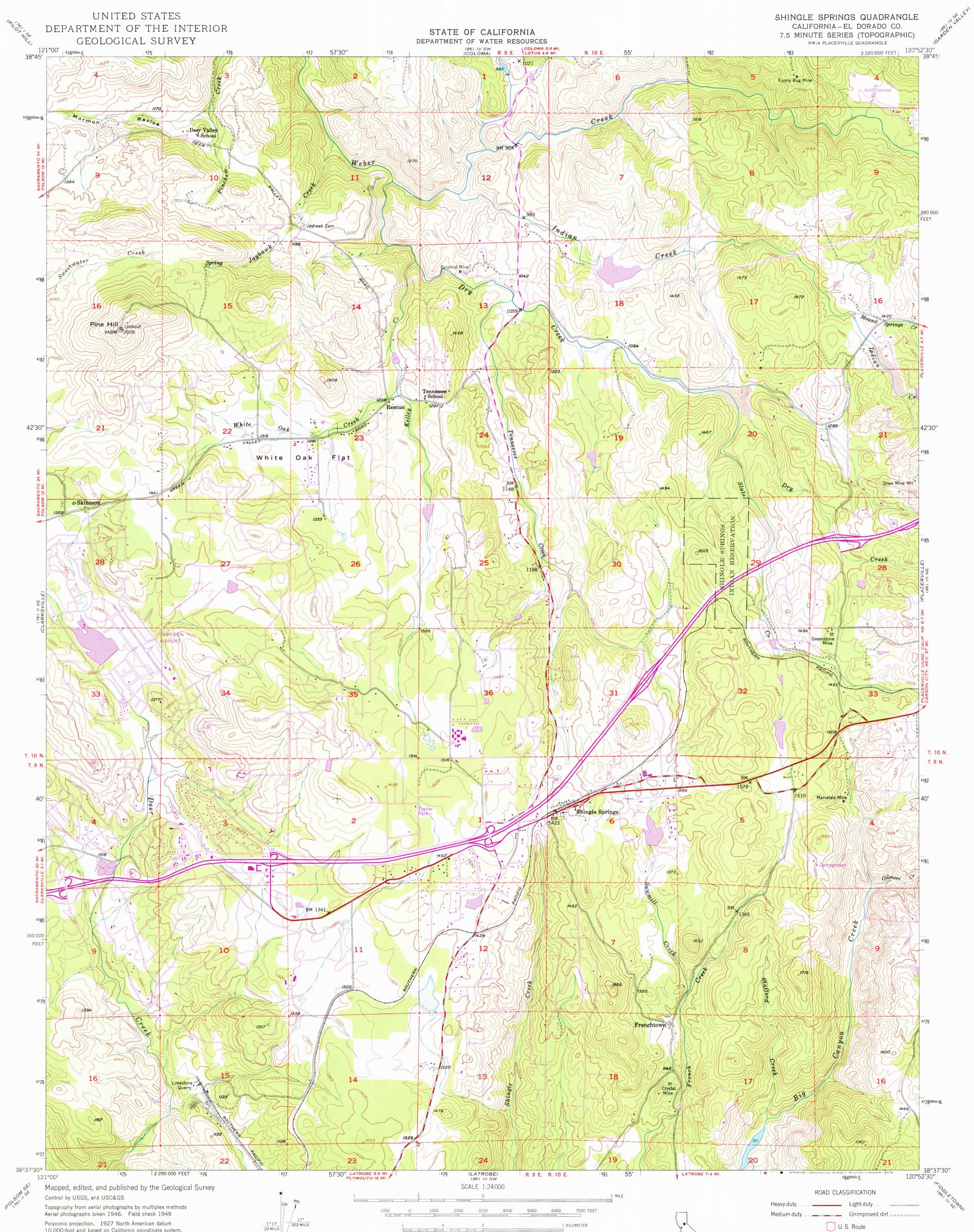
Polyconic projection. 1927 North American datum 10,000-foot grid based on California coordinate system, zone 2 1000-meter Universal Transverse Mercator grid ticks, zone 10, shown in blue Dashed land lines indicate approximate location Unchecked elevations are shown in brown Revisions shown in purple compiled from aerial photographs taken 1973. This information not field checked
