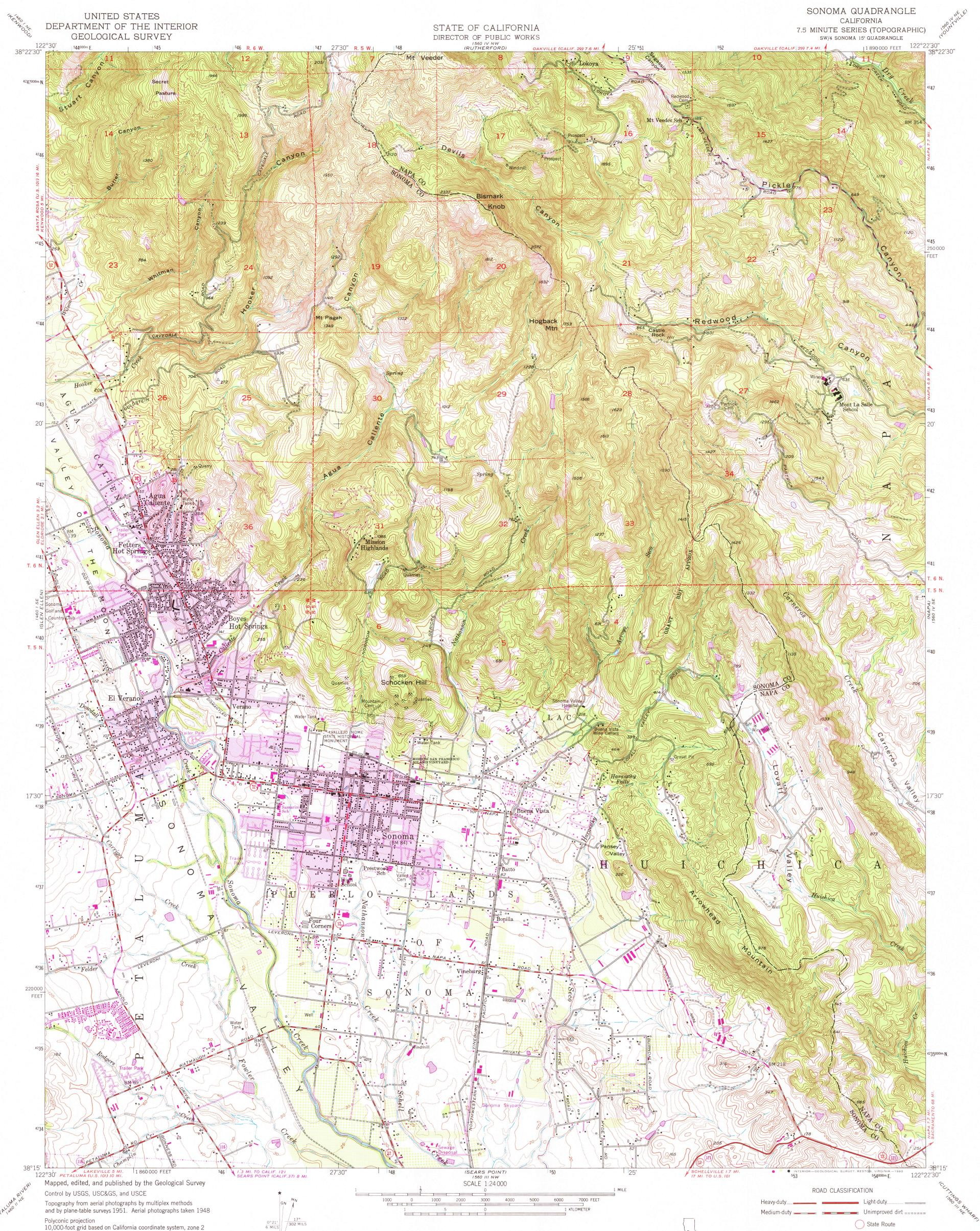
10,000-foot grid based on California coordinate system, zone 2 1000-meter Universal Transverse Mercator grid ticks, zone 10, shown in blue. 1927 North American Datum To place on the predicted North American Datum 1983 move the projection lines 15 meters north and 95 meters east as shown by dashed corner ticks
