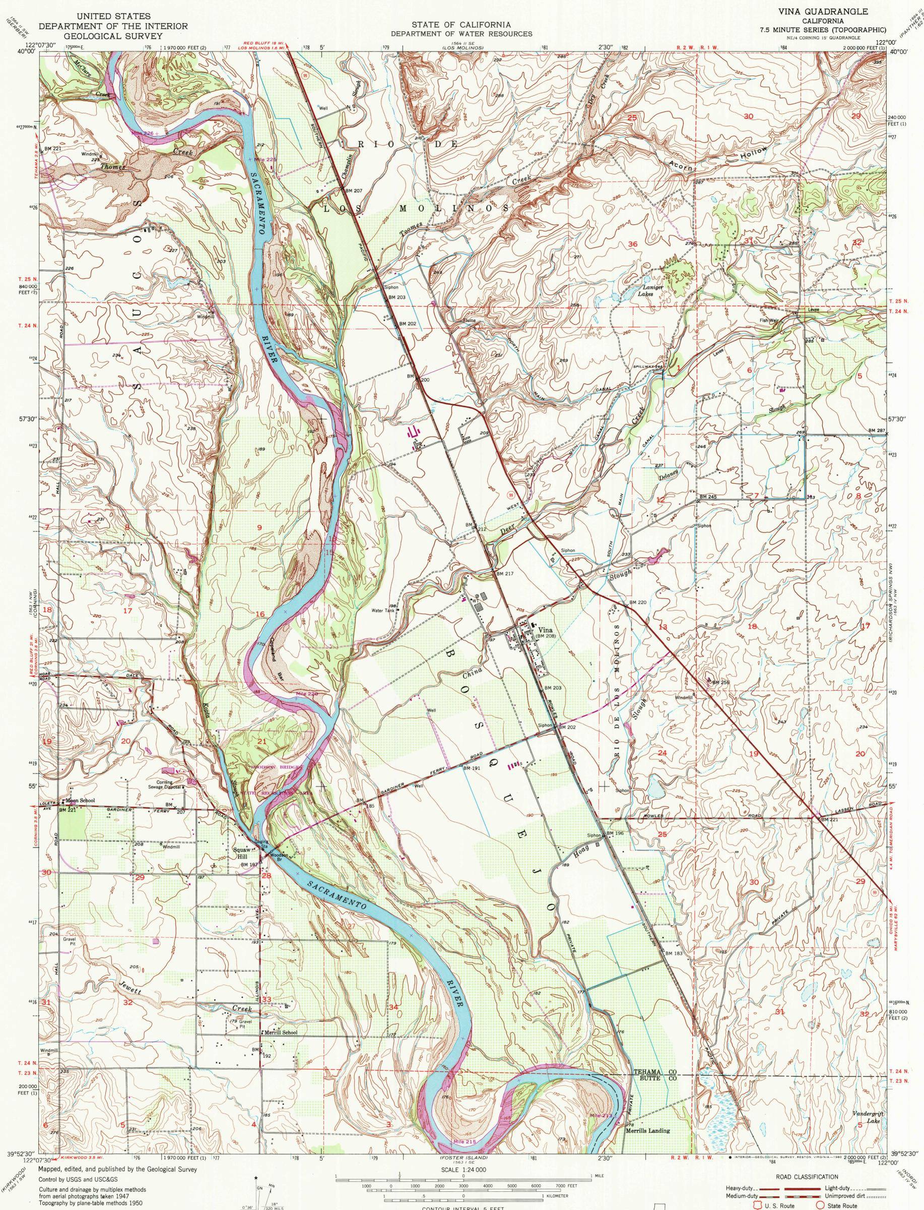
Polyconic projection. 1927 North American datum 10,000-foot grid based on California coordinate system, zones 1 and 2 1000-meter Universal Transverse Mercator grid ticks, zone 10, shown in blue. To place on the predicted North American Datum 1983 move the projection lines 17 meters north and 92 meters east as shown by dashed corner ticks There may be private inholdings within the boundaries of the National or State reservations shown on this map
