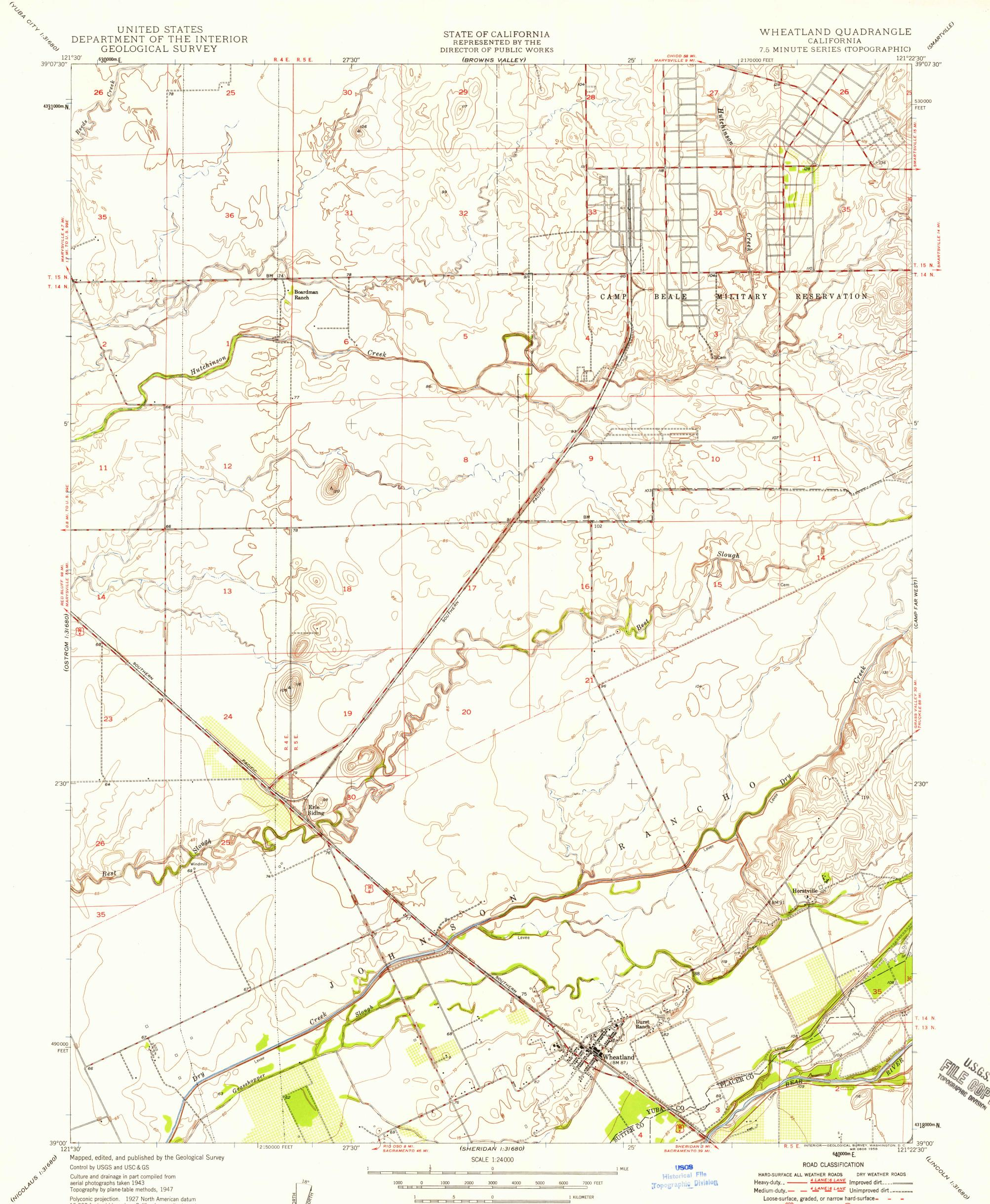
Topography by plane-table methods, 1947 Polyconic projection. 1927 North American datum 10,000-foot grid based on California coordinate system, zone 2
