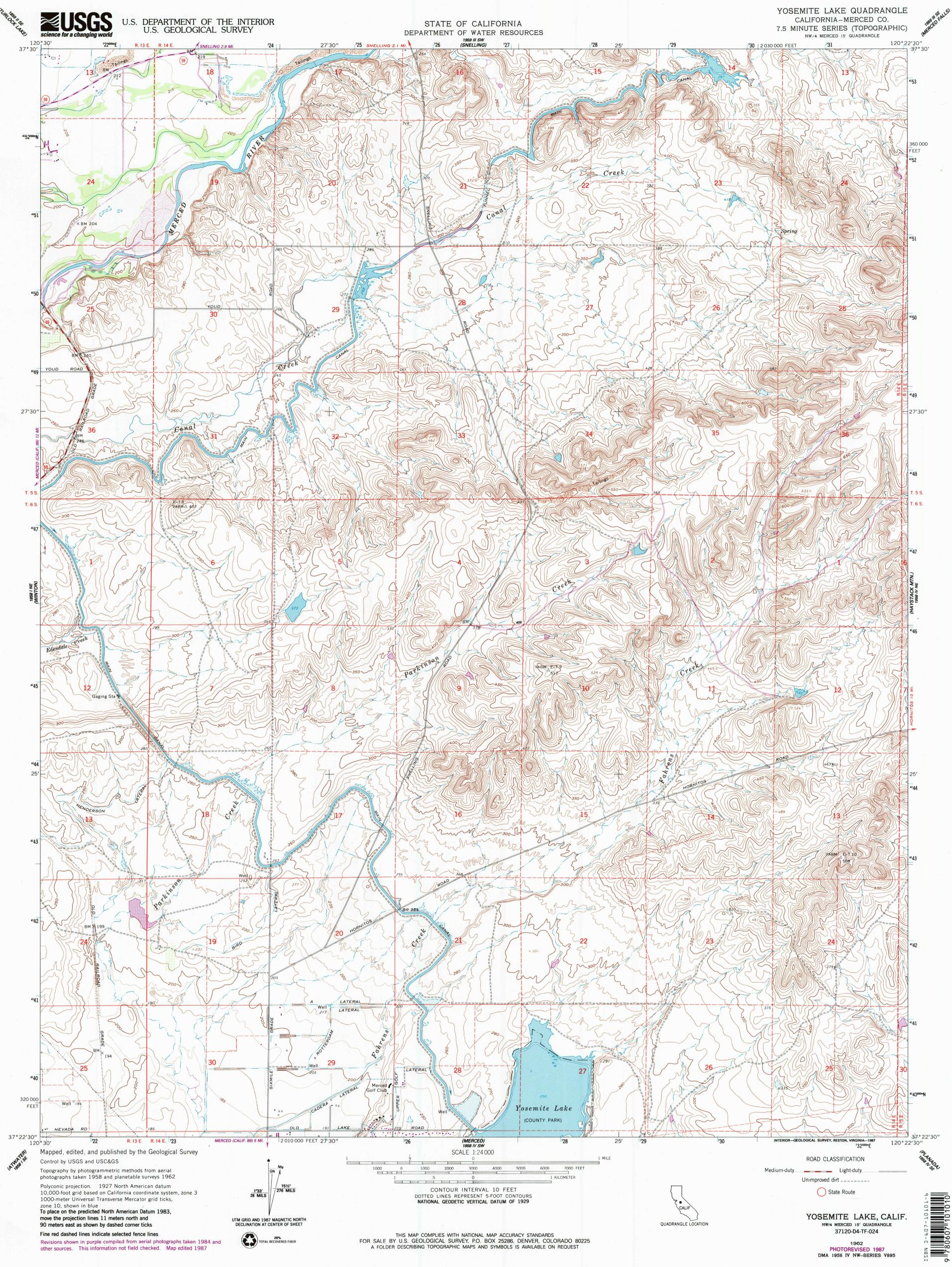
10,000-foot grid based on California coordinate system, zone 3 1000-meter Universal Transverse Mercator grid ticks, zone 10, shown in blue To place on the predicted North American Datum 1983, move the projection lines 11 meters north and 90 meters east as shown by dashed corner ticks Fine red dashed lines indicate selected fence lines Revisions shown in purple compiled from aerial photographs taken 1984 and other sources. This information not field checked. Map edited 1987
