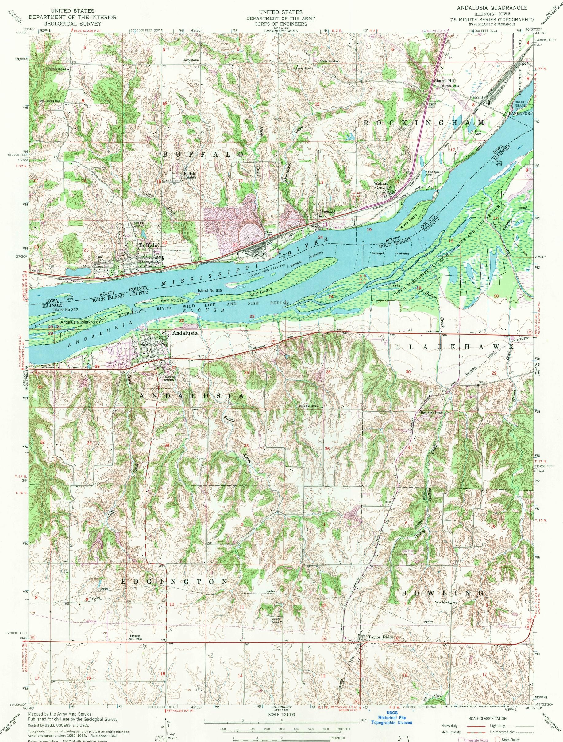
Polyconic projection. 1927 North American datum 10,000-foot grids based on Illinois coordinate system, west zone, and lowa coordinate system, south zone 1000-meter Universal Transverse Mercator grid ticks, zone 15, shown in blue
