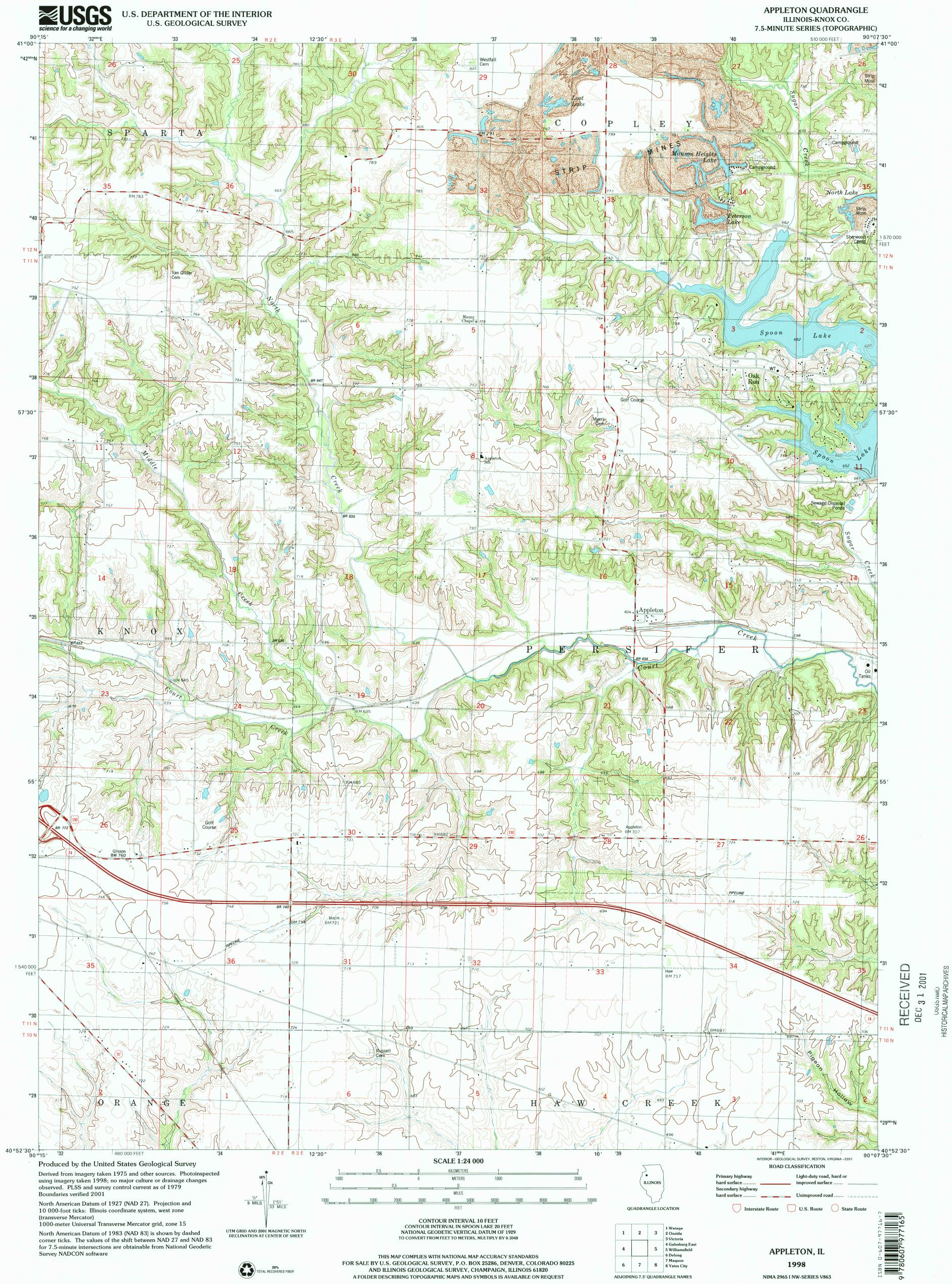
10 000-foot ticks: Illinois coordinate system, west zone (transverse Mercator) 1000-meter Universal Transverse Mercator grid, zone 15 UTM GRID AND 2001 MAGNETIC NORTH DECLINATION AT CENTER OF SHEET North American Datum of 1983 (NAD 83) is shown by dashed corner ticks. The values of the shift between NAD 27 and NAD 83 for 7.5-minute intersections are obtainable from National Geodetic Survey NADCON software
