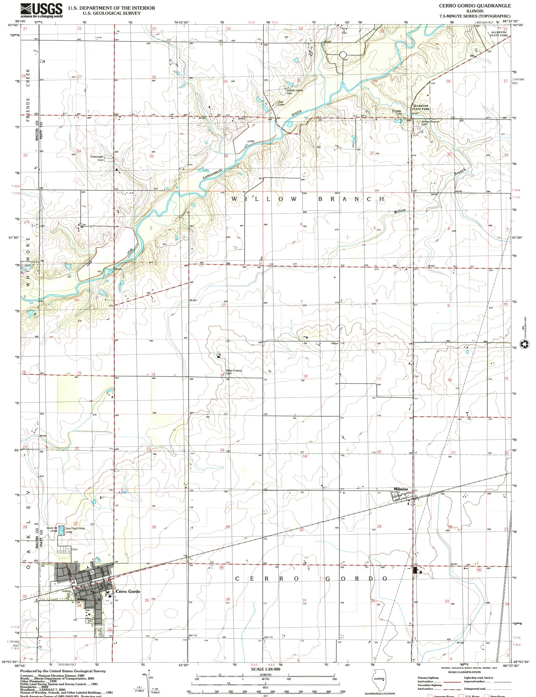
North American Datum of 1983 (NAD 83). Projection and 1 000-meter grid: Universal Transverse Mercator, zone 16S 10 000-foot ticks: Illinois Coordinate System of 1983 (east zone)
