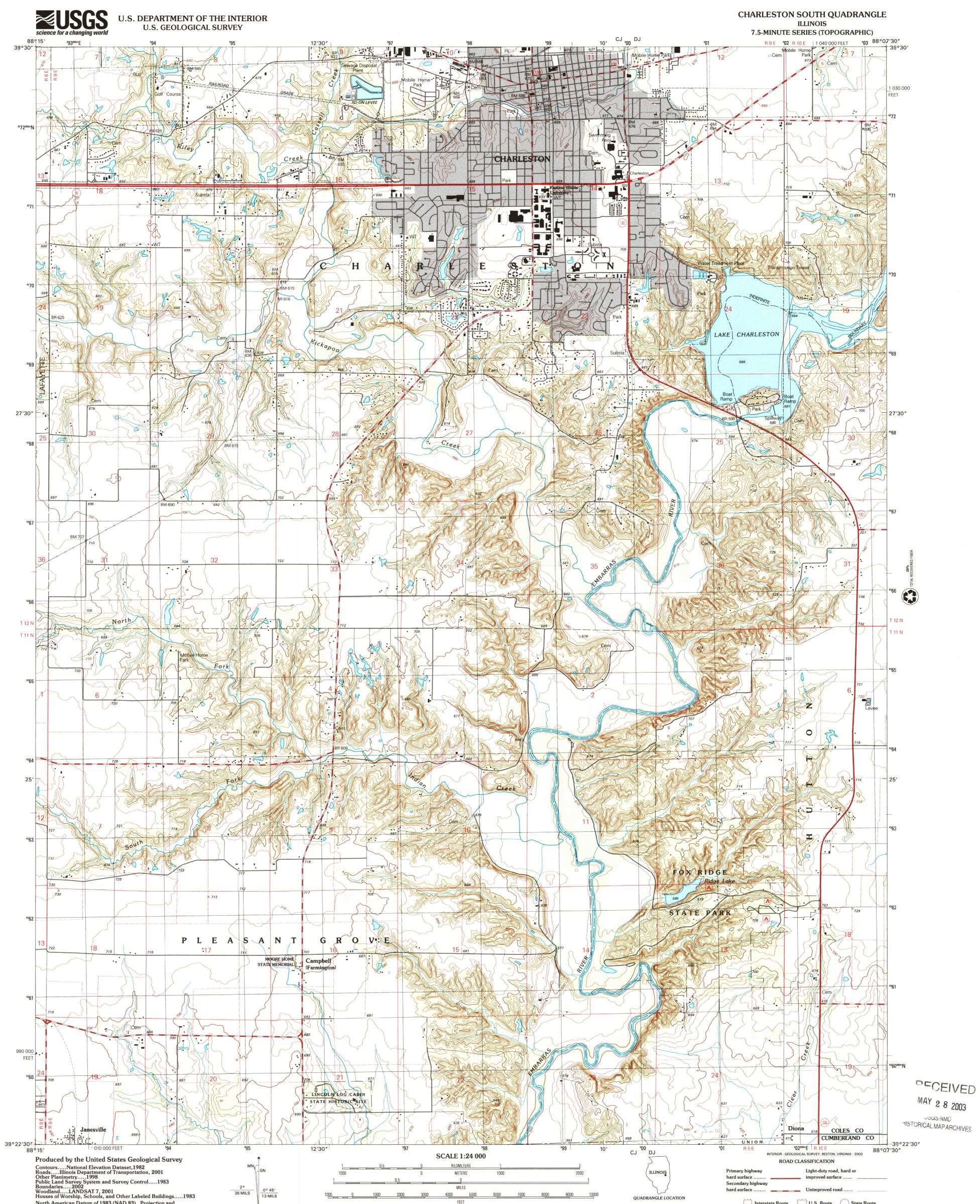
North American Datum of 1983 (NAD 83). Projection and 1 000-meter grid: Universal Transverse Mercator, zone 16S 10 000-foot ticks: Illinois Coordinate System of 1983 (east zone) North American Datum of 1927 (NAD 27) is shown by dashed corner ticks. The values of the shift between NAD 83 and NAD 27 for 7.5-minute intersections are obtainable from National Geodetic Survey NADCON software There may be private inholdings within the boundaries of the National or State reservations shown on this map
