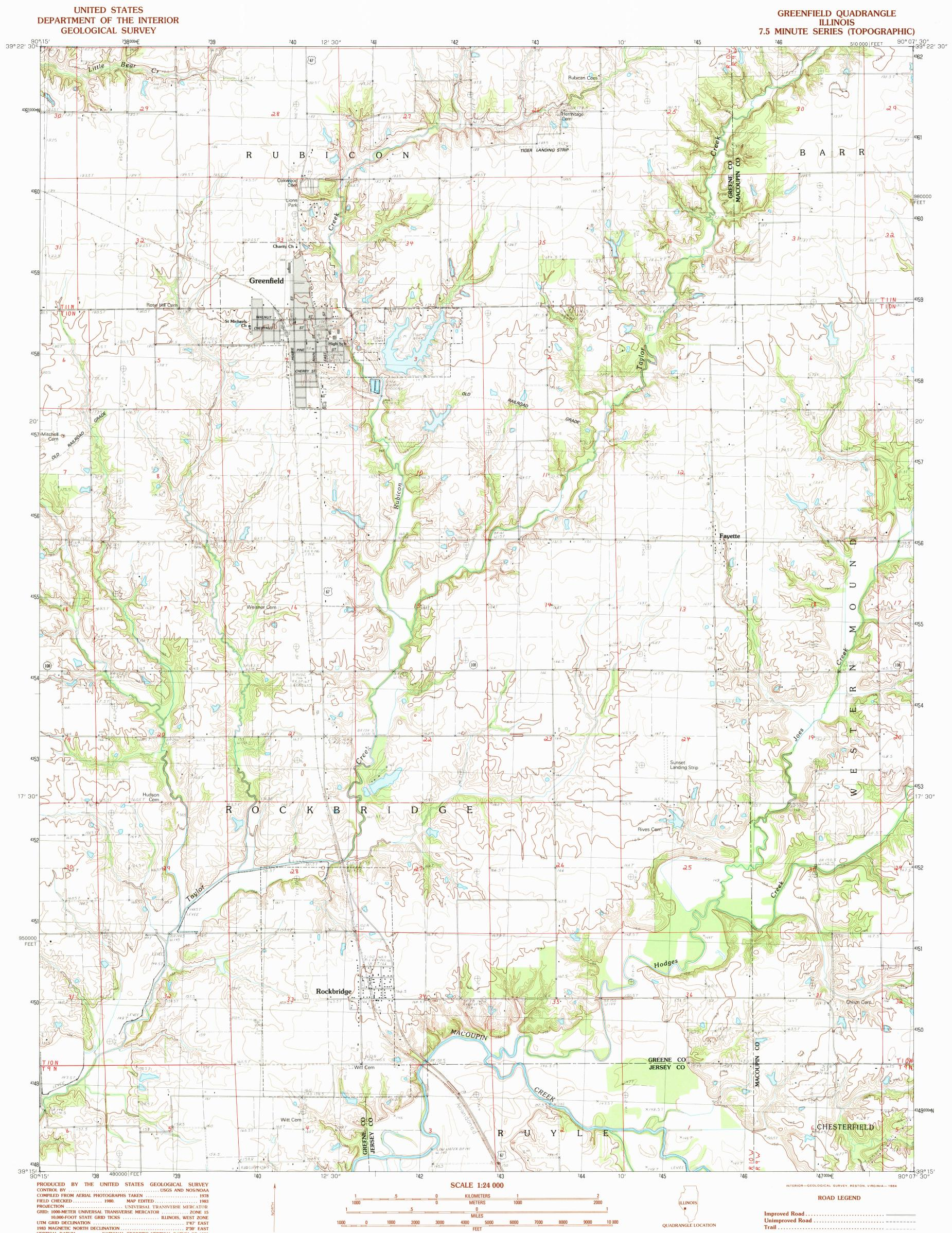
UTM GRID DECLINATION ... . 1°47' EAST 1983 MAGNETIC NORTH DECLINATION ..... ... 2°30' EAST To place on the predicted North American Datum of 1983 move the projection lines as shown by dashed corner ticks (1 meter south and 9 meters east) There may be private inholdings within the boundaries of any Federal and State reservations shown on this map Gray tint indicates area in which selected buildings are shown
