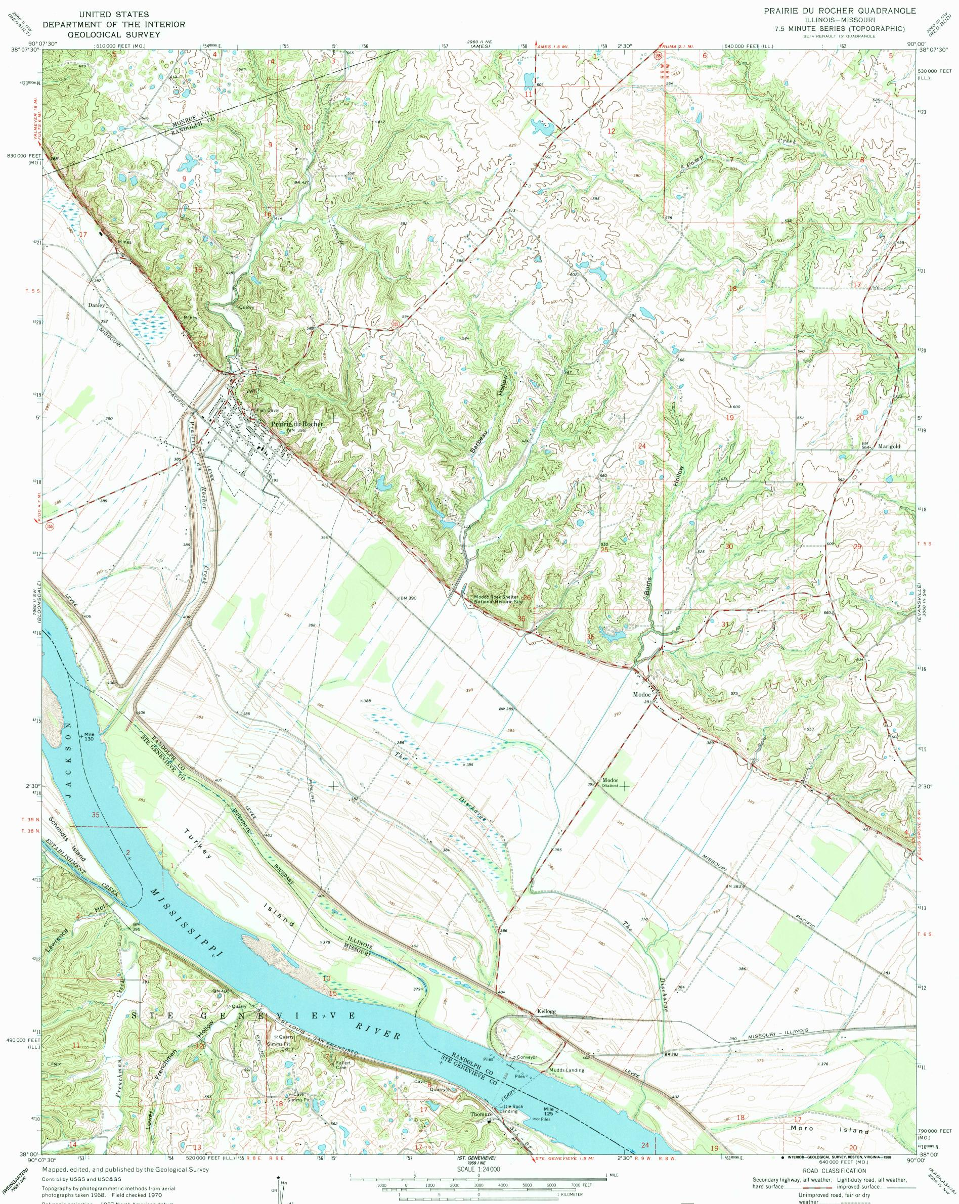
Polyconic projection. 1927 North American datum 10,000-foot grids based on Illinois coordinate system, west zone and Missouri coordinate system, east zone 1000-meter Universal Transverse Mercator grid ticks, zone 15, shown in blue
