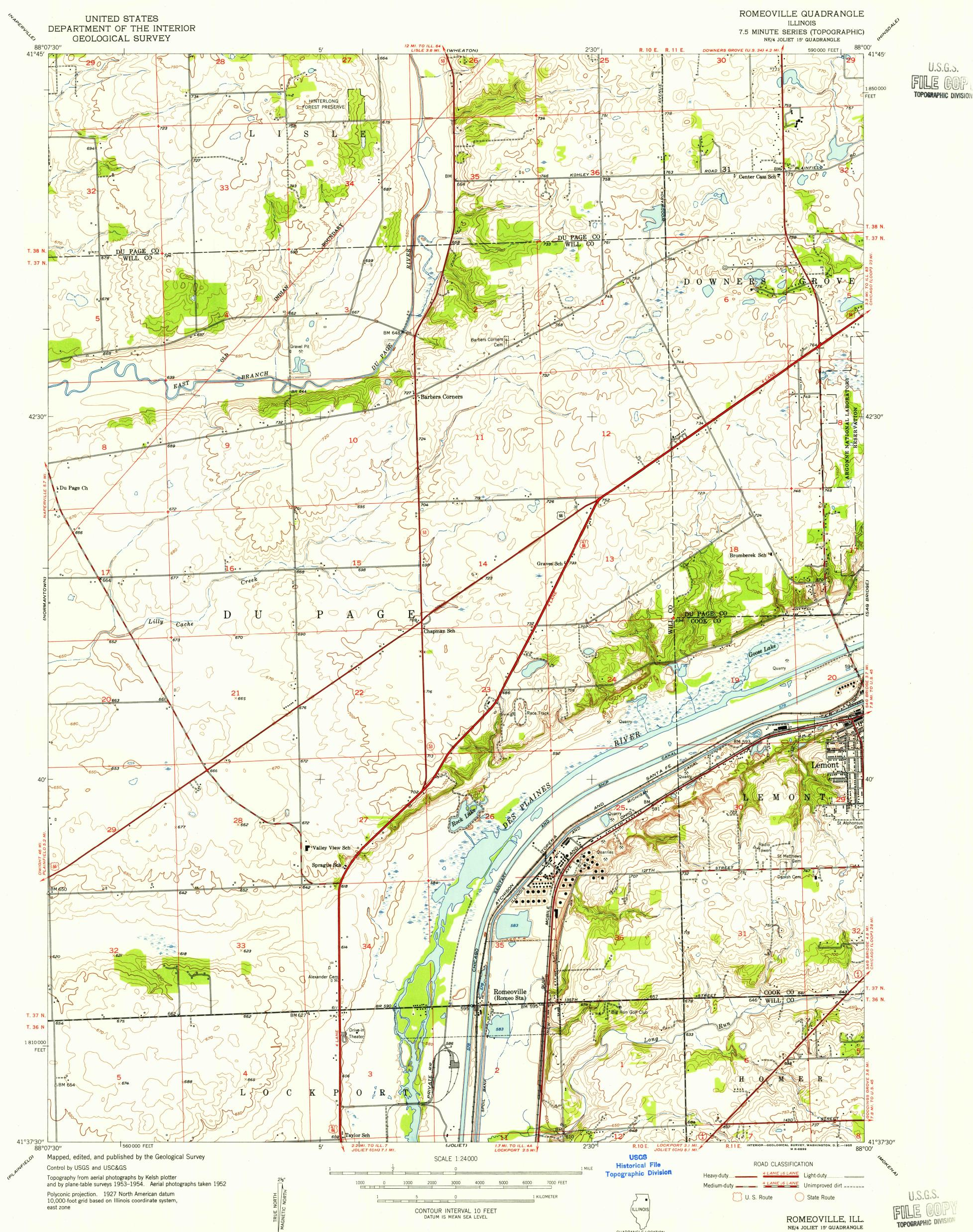
Polyconic projection. 1927 North American datum 10,000-foot grid based on Illinois coordinate system, east zone
