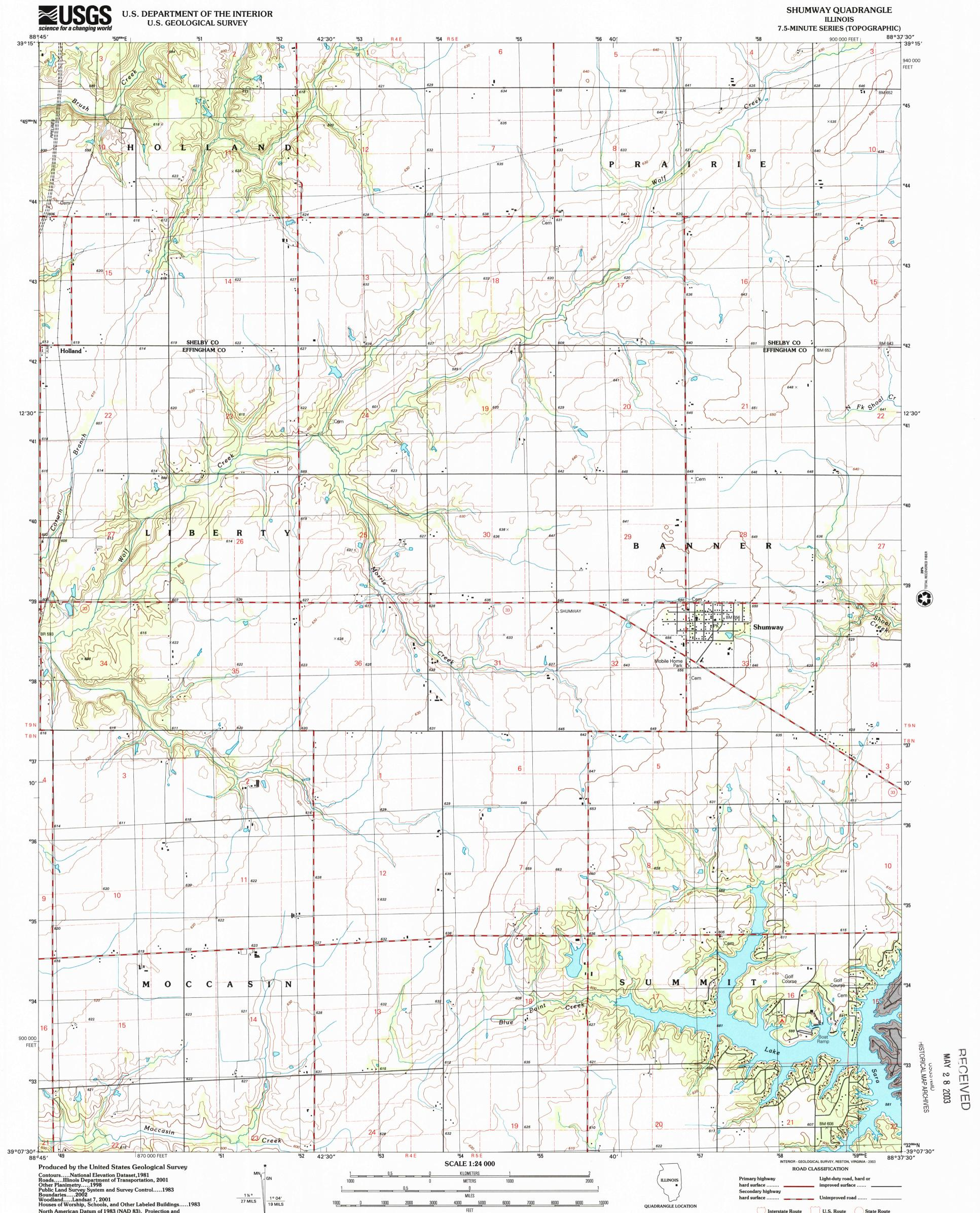
North American Datum of 1983 (NAD 83). Projection and 1 000-meter grid: Universal Transverse Mercator, zone 16S 10 000-foot ticks: Illinois Coordinate System of 1983 (east zone) North American Datum of 1927 (NAD 27) is shown by dashed corner ticks. The values of the shift between NAD 83 and NAD 27 for 7.5-minute intersections are obtainable from National Geodetic Survey NADCON software
