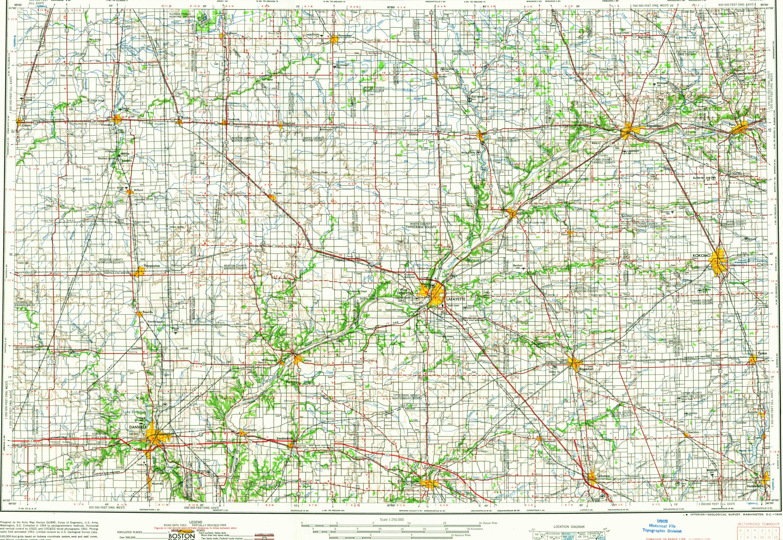
Prepared by the Army Map Service (AJBM), Corps of Engineers, U.S. Army, Washington, D.C. Compiled in 1954 by photogrammetric methods. Horizontal and vertical control by USGS. and USC&GS Aerial photography 1952. Photography field annotated 1953. Limited revision by U.S. Geological Survey 1965. 100,000-foot grids based on Indiana coordinate system, west and east zones, and Illinois coordinate system, east zone
