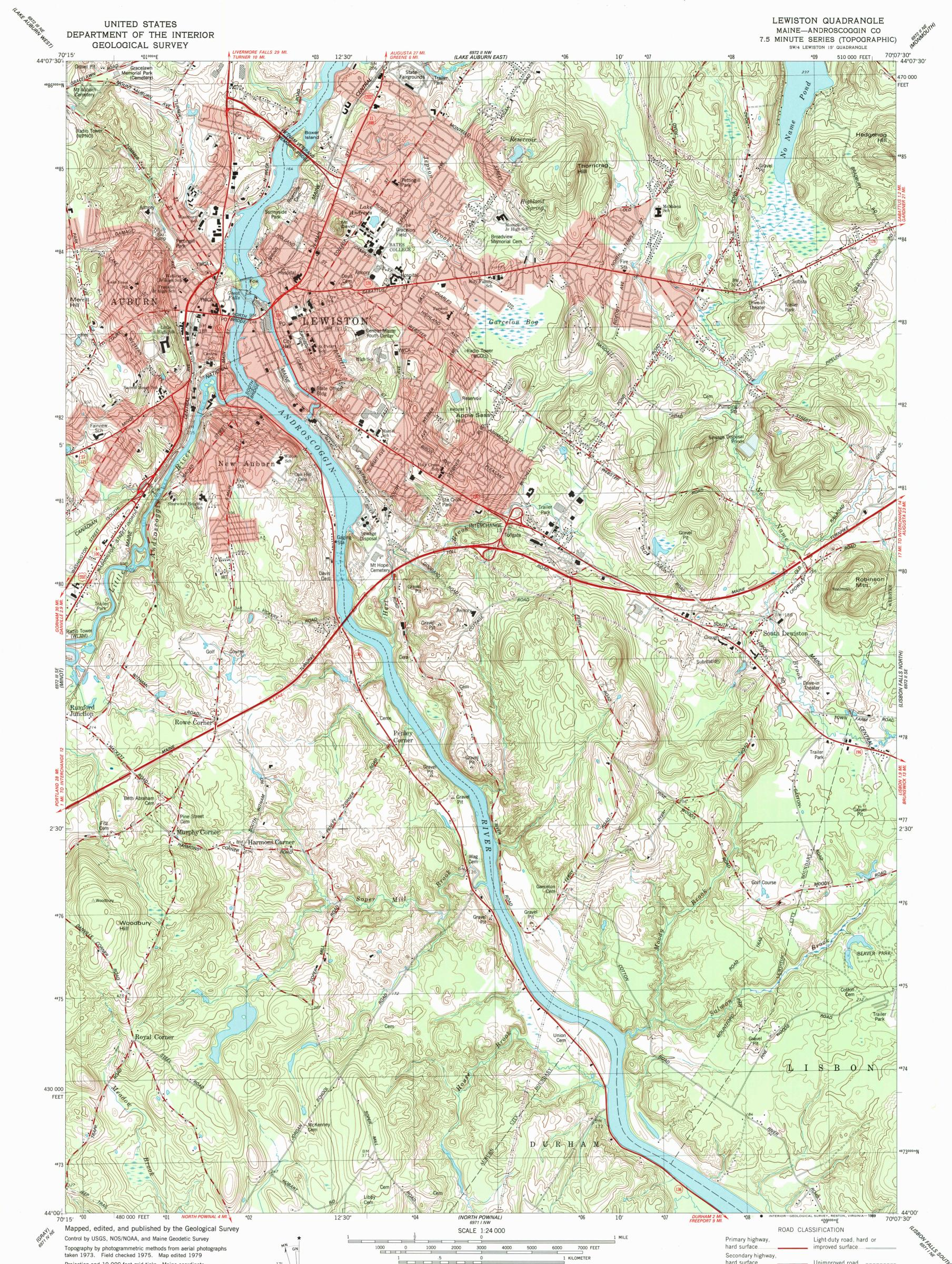
Projection and 10,000-foot grid ticks: Maine coordinate system, west zone (transverse Mercator) 1000-meter Universal Transverse Mercator grid, zone 19 1927 North American Datum To place on the predicted North American Datum 1983 move the projection lines 4 meters south and 42 meters west as shown by dashed corner ticks
