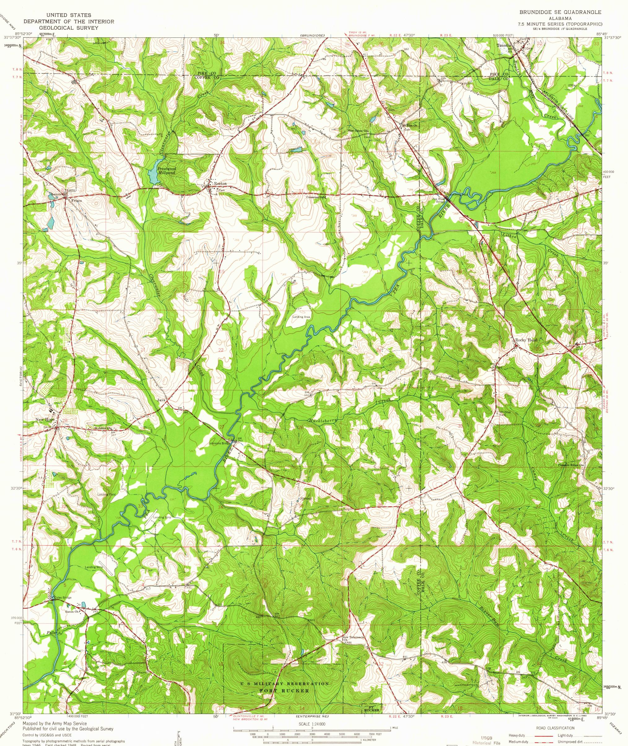
Topography by photogrammetric methods from aerial photographs taken 1946. Field checked 1948. Revised from aerial photographs taken 1959. Field checked 1960
