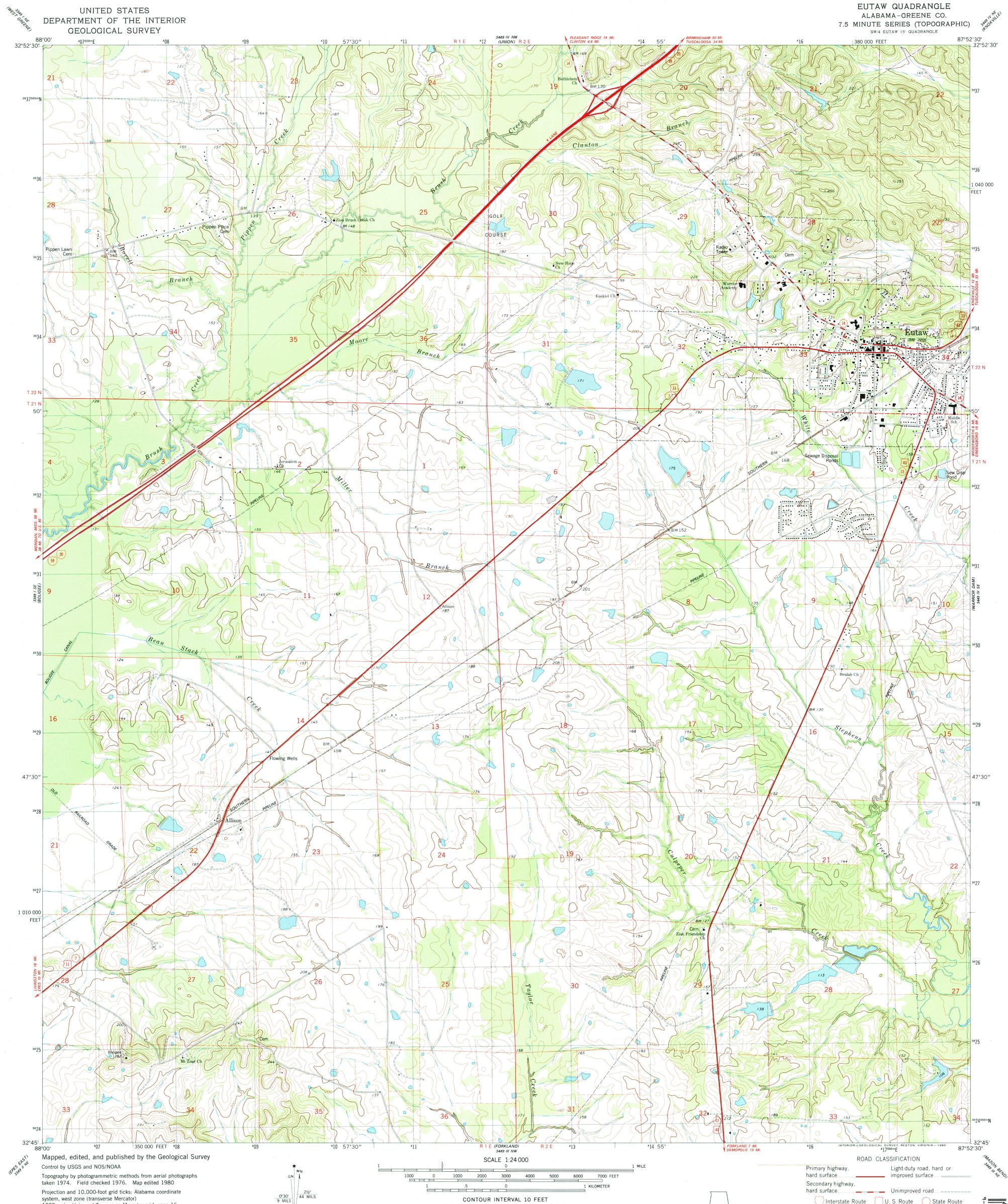
system, west zone (transverse Mercator) 1000-meter Universal Transverse Mercator grid, zone 16 1927 North American Datum To place on the predicted North American Datum 1983 move the projection lines 12 meters south and 1 meter east as shown by dashed corner ticks
