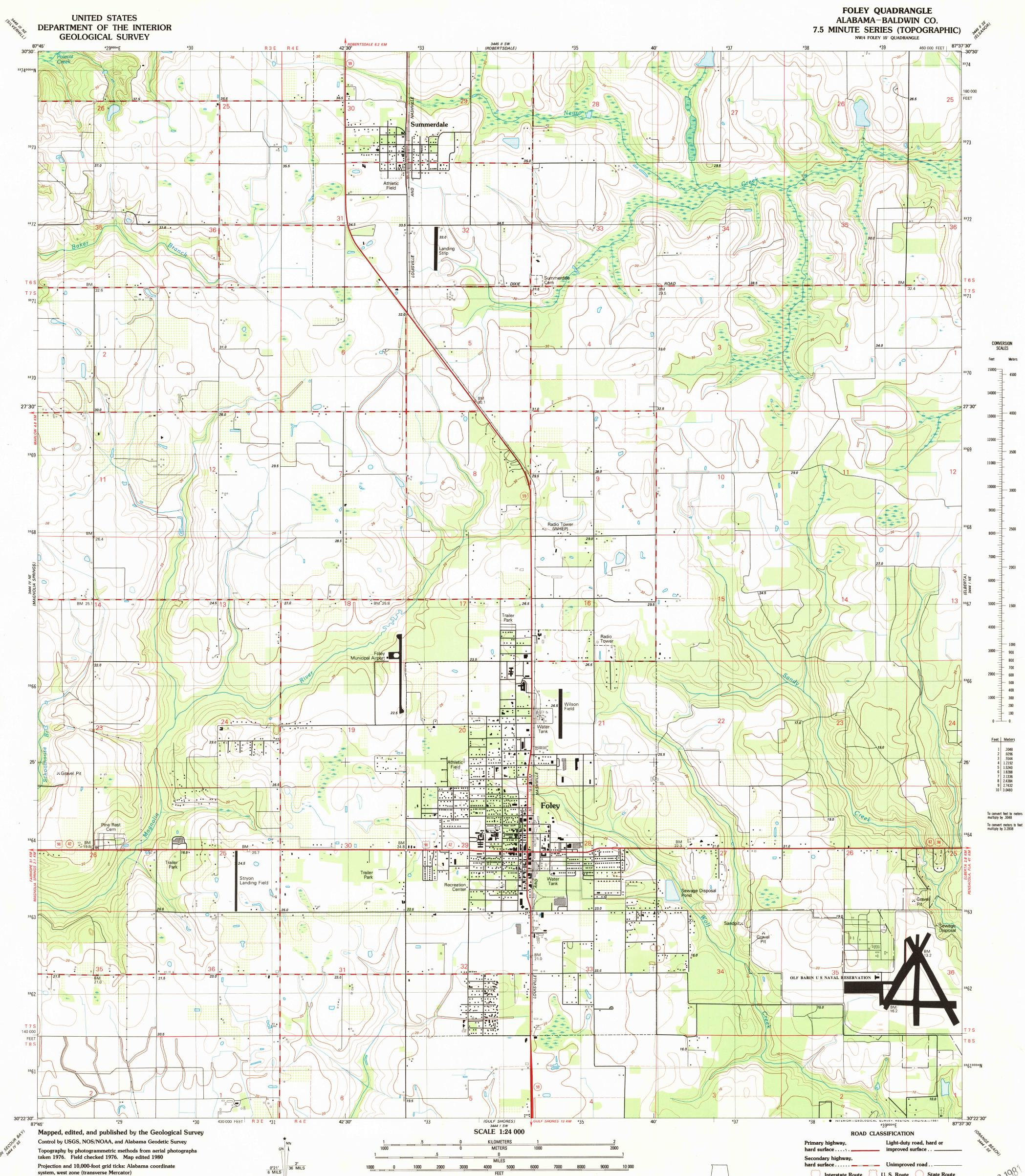
system, west zone (transverse Mercator) 1000-meter Universal Transverse Mercator grid, zone 16 1927 North American Datum To place on the predicted North American Datum 1983 move the projection lines 18 meters south and 1 meter west as shown by dashed corner ticks
