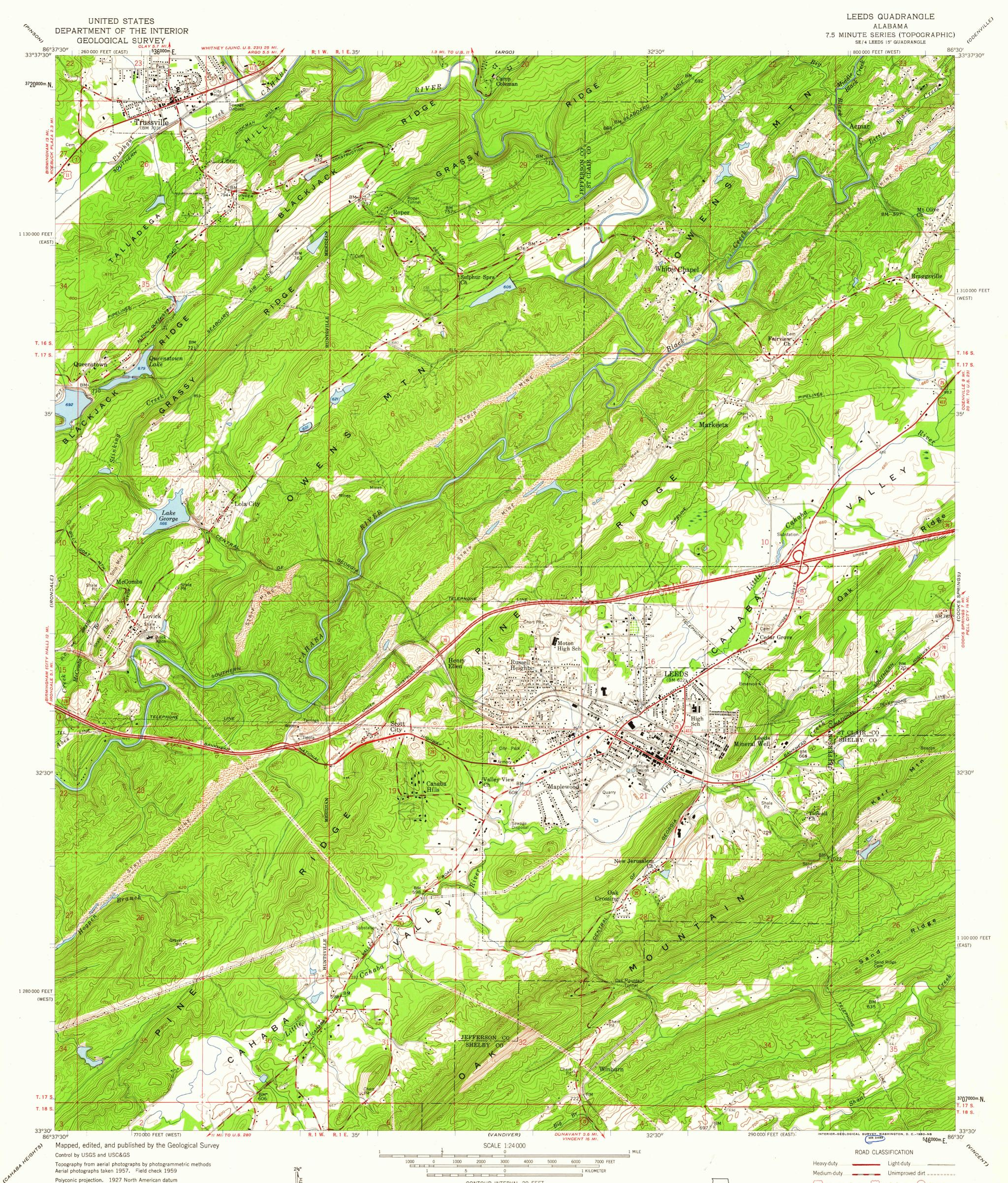
Polyconic projection. 1927 North American datum 10,000-foot grids based on Alabama coordinate system, west and east zones 1000-meter Universal Transverse Mercator grid ticks, zone 16, shown in blue Unchecked elevations are shown in brown
