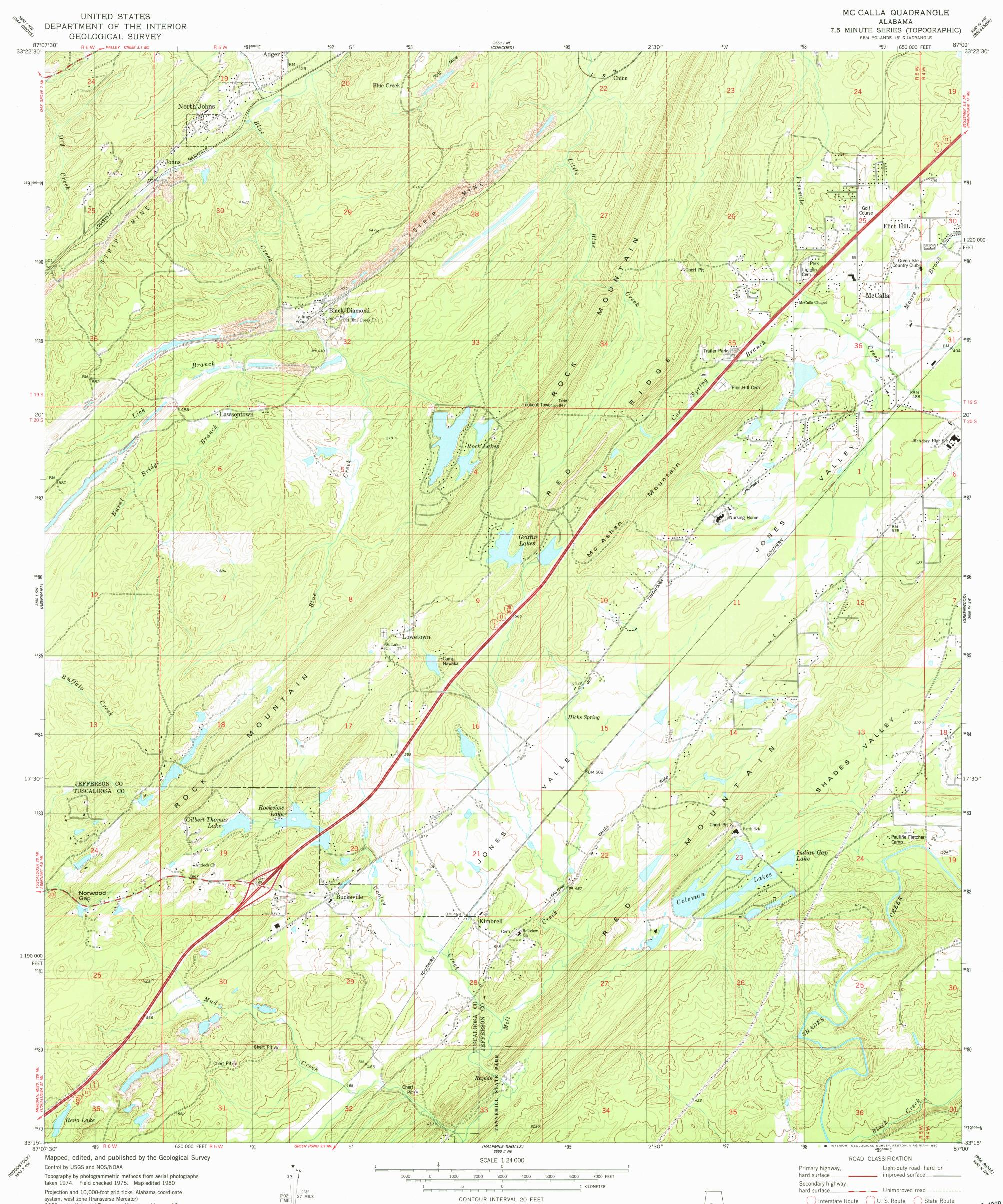
system, west zone (transverse Mercator) 1000-meter Universal Transverse Mercator grid, zone 16 1927 North American Datum To place on the predicted North American Datum 1983 move the projection lines 10 meters south and 1 meter west as shown by dashed corner ticks
