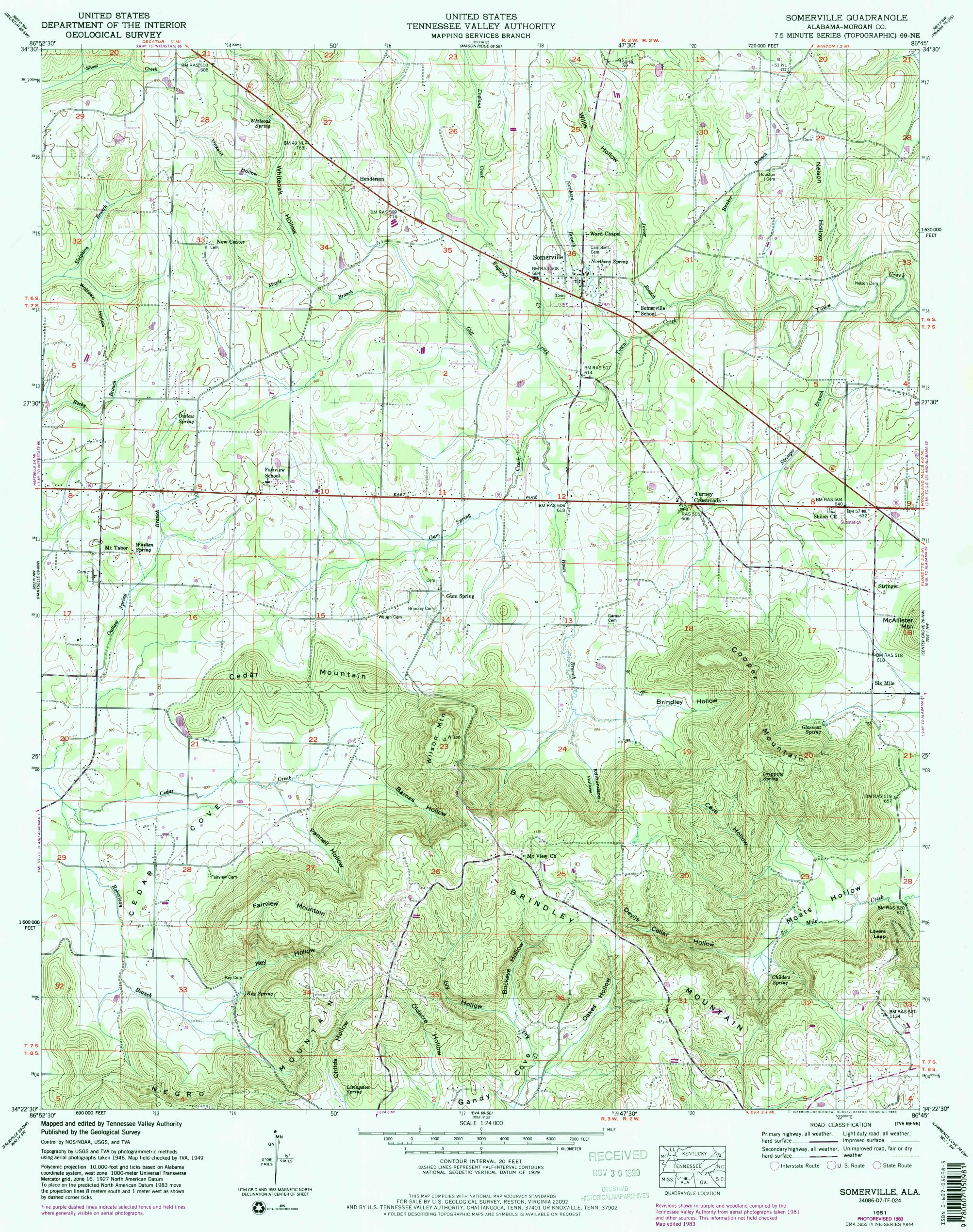
Polyconic projection. 10,000-foot grid ticks based on Alabama coordinate system, west zone. 1000-meter Universal Transverse Mercator grid, zone 16. 1927 North American Datum To place on the predicted North American Datum 1983 move the projection lines 8 meters south and 1 meter west as shown by dashed corner ticks
