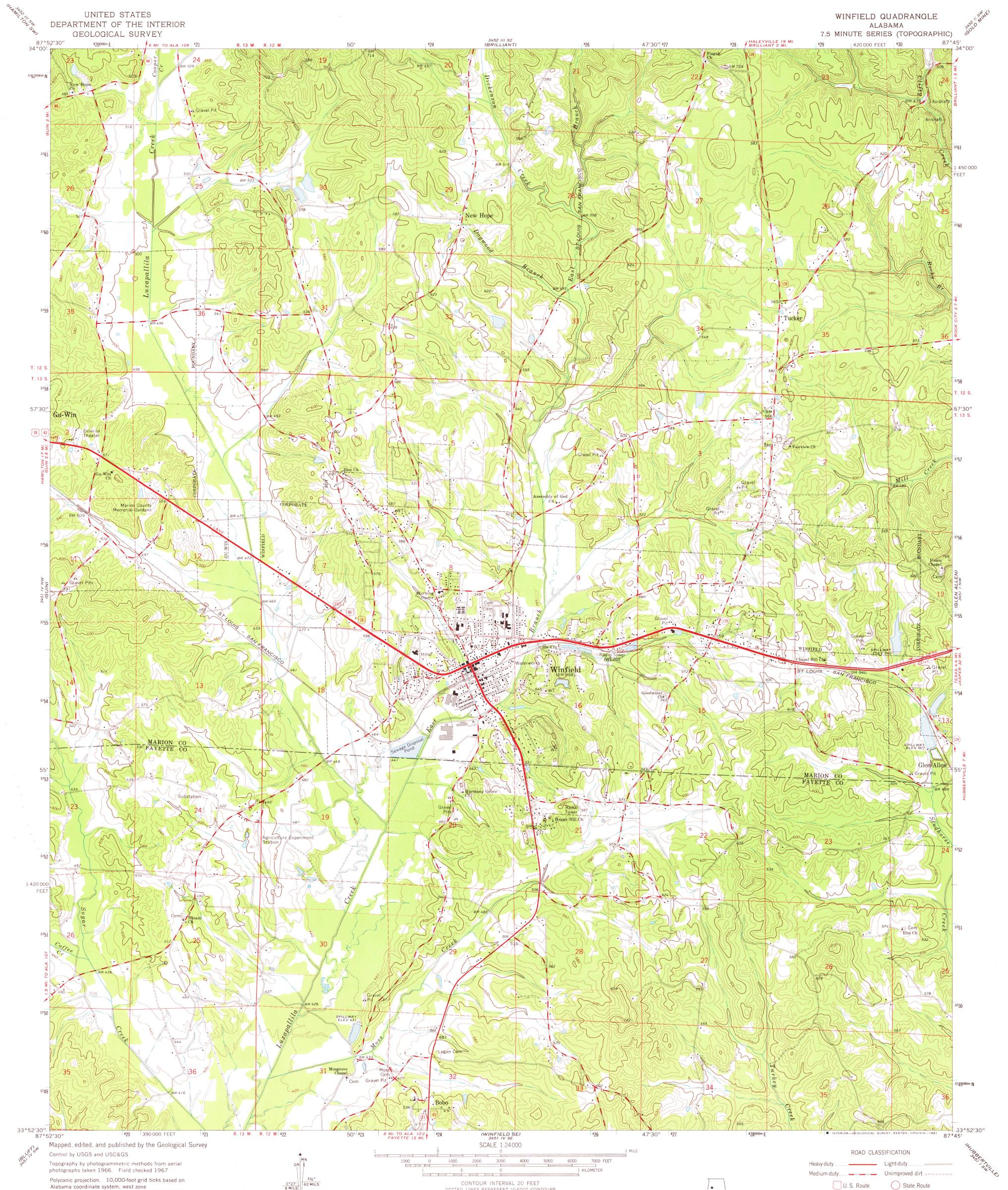
1000-meter Universal Transverse Mercator grid ticks, zone 16, shown in blue. 1927 North American Datum To place on the predicted North American Datum 1983 move the projection lines 9 meters south and 2 meters east as shown by dashed corner ticks
