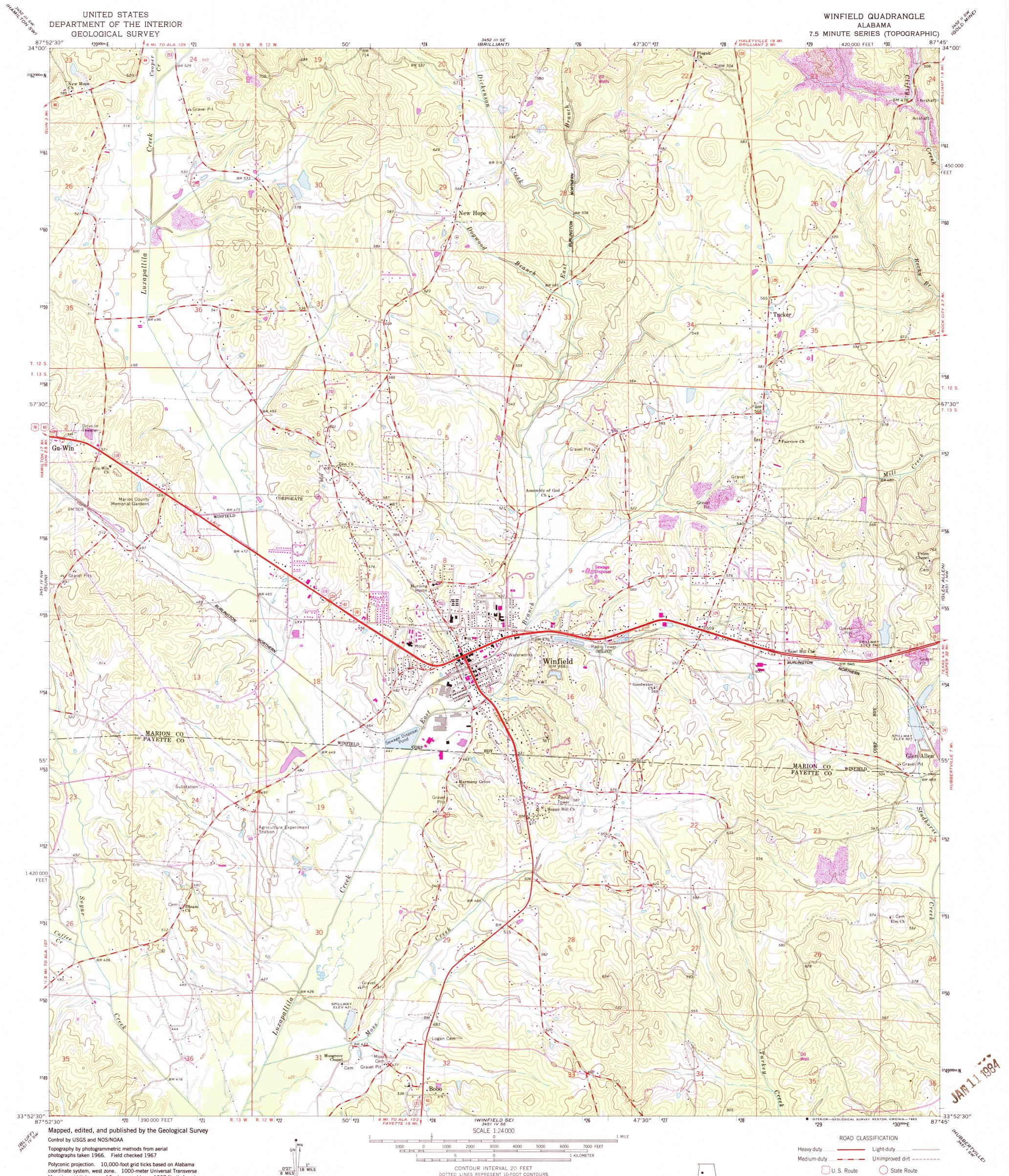
Mercator grid ticks, zone 16, shown in blue. 1927 North American Datum. To place on the predicted North American Datum 1983 move the projection lines 9 meters south and 2 meters east as shown by dashed corner ticks
