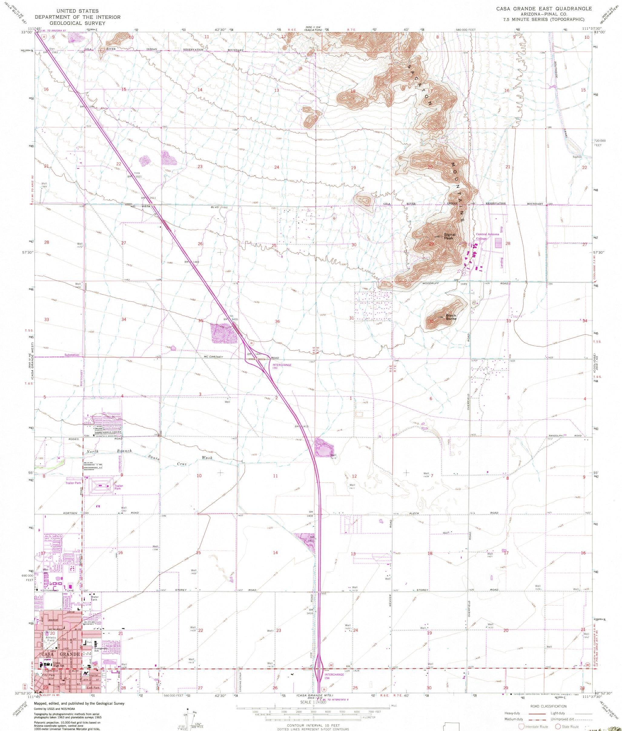
1000-meter Universal Transverse Mercator grid ticks, zone 12, shown in blue. 1927 North American Datum To place on the predicted North American Datum 1985 move the projection lines 3 meters south and 63 meters east as shown by dashed corner ticks
