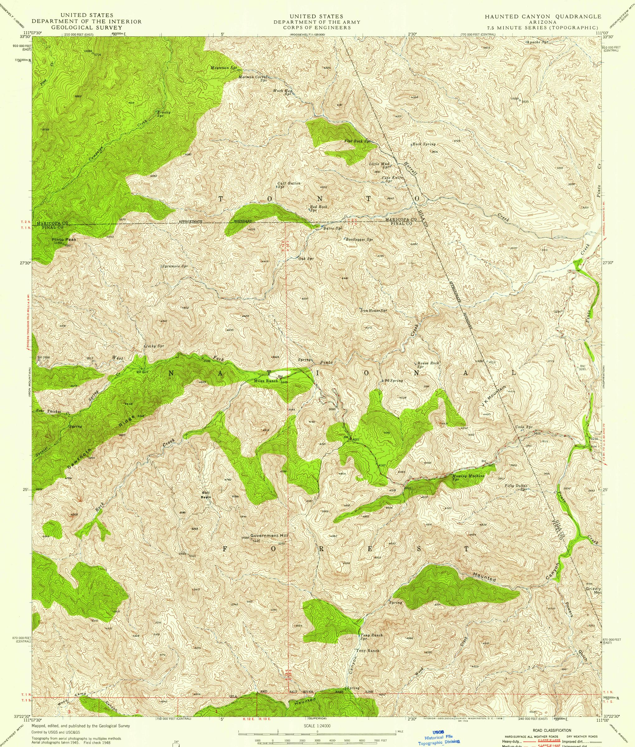
Polyconic projection. 1927 North American datum 10,000-foot grid based on Arizona coordinate system, central and east zones.
