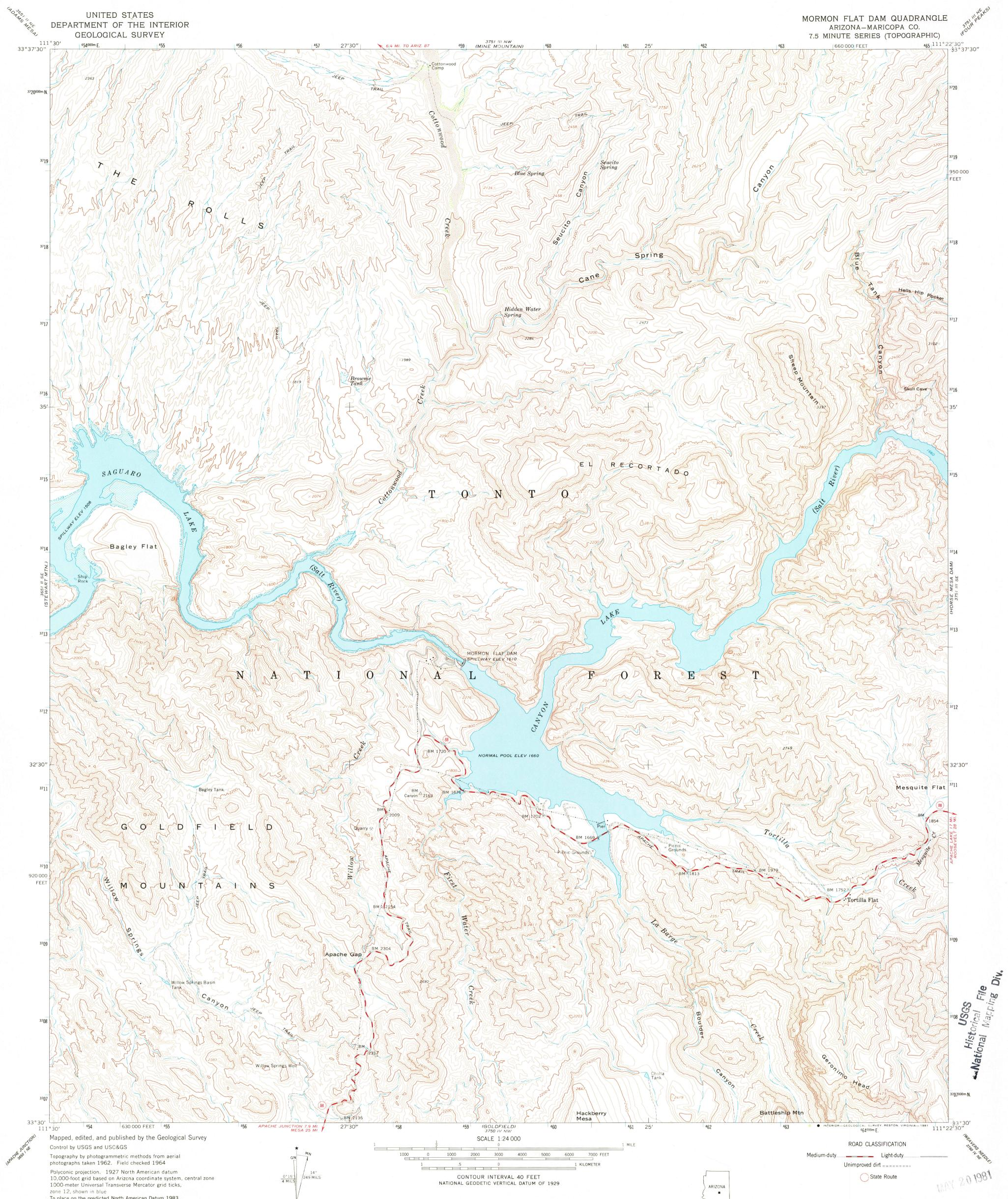
Polyconic projection. 1927 North American datum 10,000-foot grid based on Arizona coordinate system, central zone 1000-meter Universal Transverse Mercator grid ticks, zone 12, shown in blue To place on the predicted North American Datum 1983 move the projection lines 2 meters south and 63 meters east as shown by dashed corner ticks Areas covered by dashed light blue pattern are subject to controlled inundation
