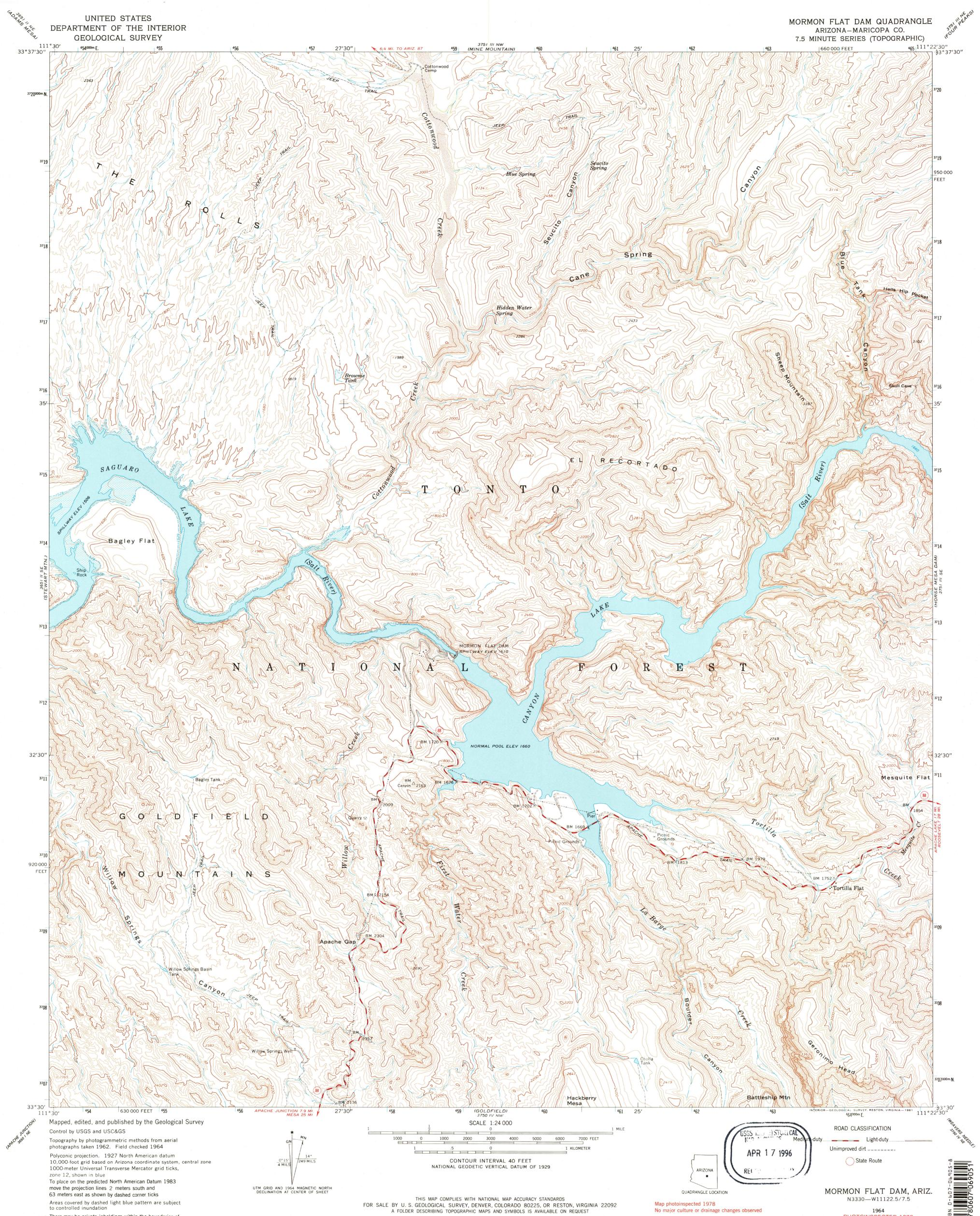
10,000-foot grid based on Arizona coordinate system, central zone 1000-meter Universal Transverse Mercator grid ticks, zone 12, shown in blue To place on the predicted North American Datum 1983 move the projection lines 2 meters south and 63 meters east as shown by dashed corner ticks Areas covered by dashed light blue pattern are subject to controlled inundation
