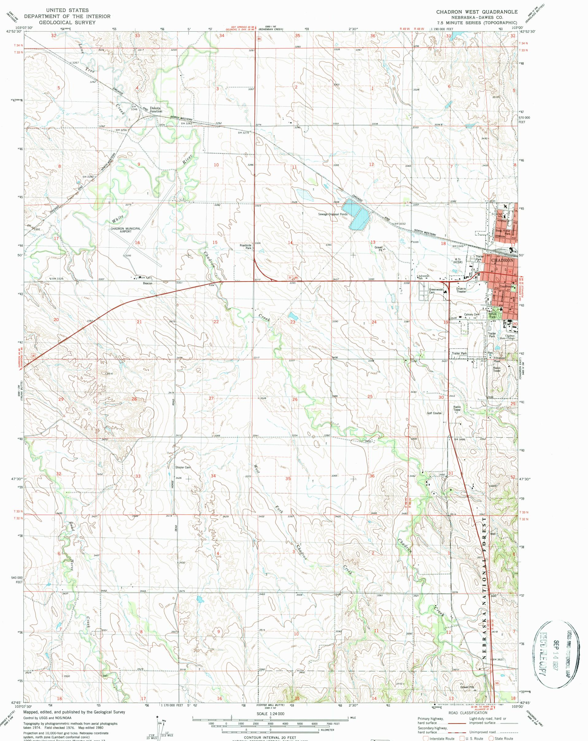
Projection and 10,000-foot grid ticks: Nebraska coordinate system, north zone (Lambert conformal conic) 1000-meter Universal Transverse Mercator grid, zone 13 1927 North American Datum To place on the predicted North American Datum 1983 move the projection lines 6 meters north and 42 meters east as shown by dashed corner ticks
