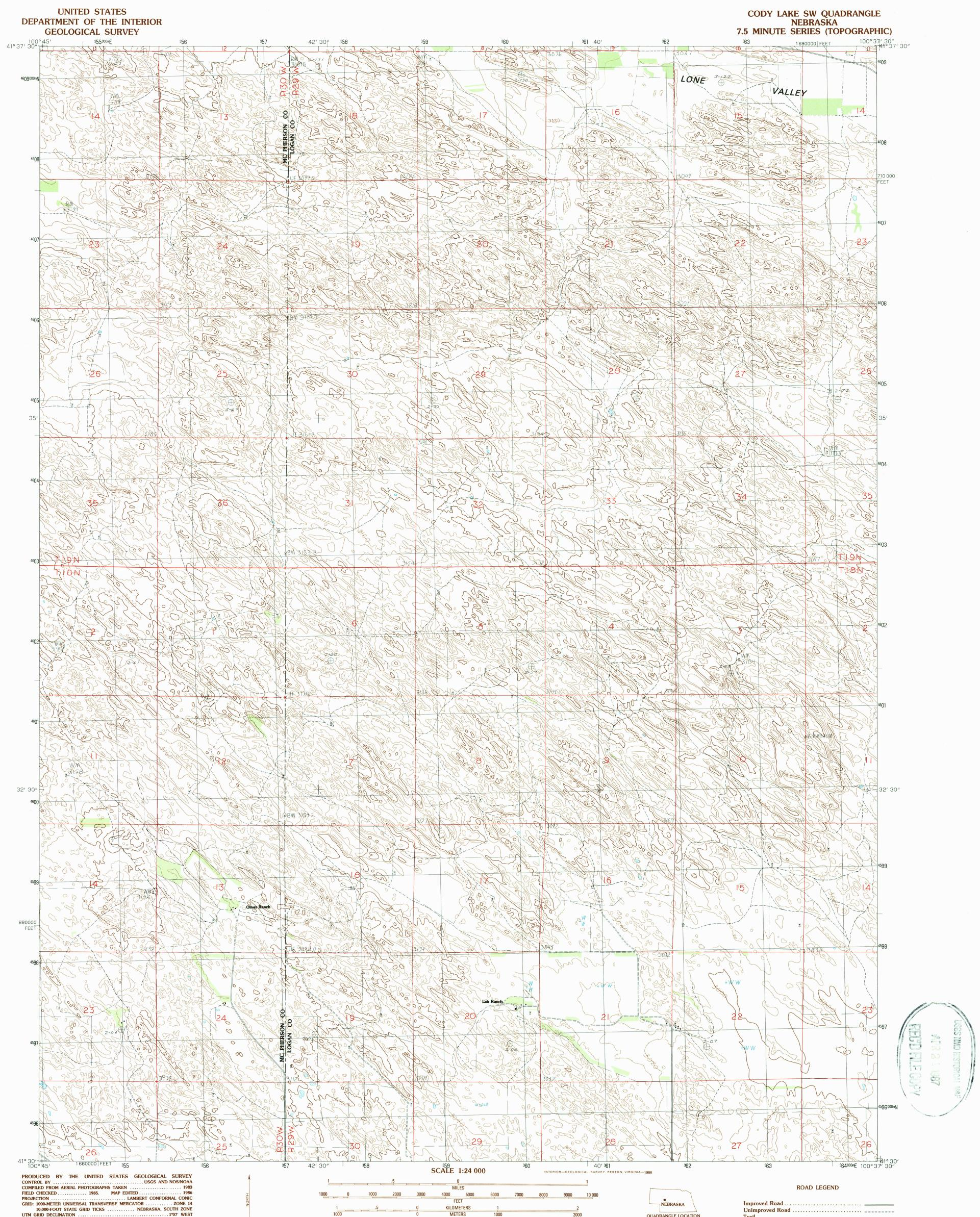
PROVISIONAL MAP Produced from original manuscript drawings. Information shown as of date of photography. 1 CONTOUR INTERVAL 20 FEET SUPPLEMENTARY CONTOUR INTERVAL 10 FEET CONTROL ELEVATIONS SHOWN TO THE NEAREST 0.1 FOOT OTHER ELEVATIONS SHOWN TO THE NEAREST FOOT To convert feet to meters multiply by .3048 To convert meters to feet multiply by 3.2808 THIS MAP COMPLIES WITH NATIONAL MAP ACCURACY STANDARDS FOR SALE BY U. S. GEOLOGICAL SURVEY DENVER, COLORADO 80225, OR RESTON, VIRGINIA 22092
