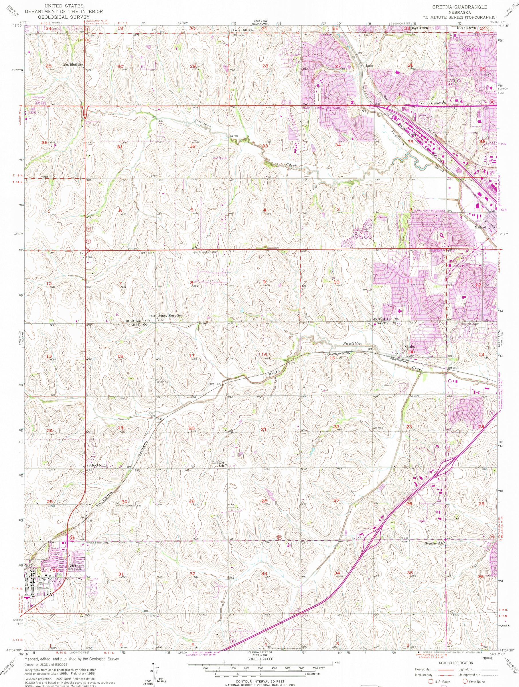
Polyconic projection. 1927 North American datum 10,000-foot grid based on Nebraska coordinate system, south zone 1000-meter Universal Transverse Mercator grid ticks, zone 14, shown in blue
