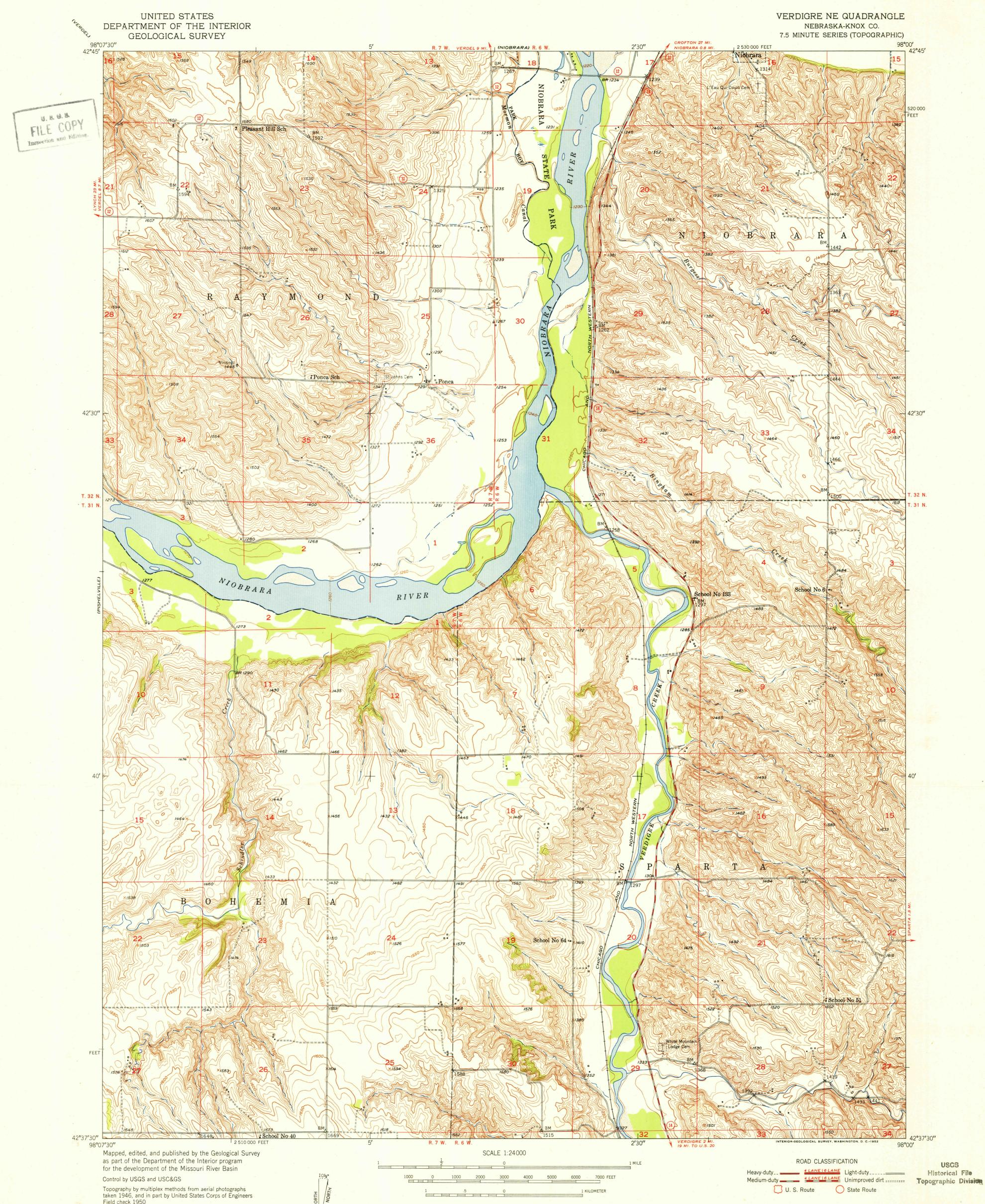
Topography by multiplex methods from aerial photographs taken 1946, and in part by United States Corps of Engineers Field check 1950
