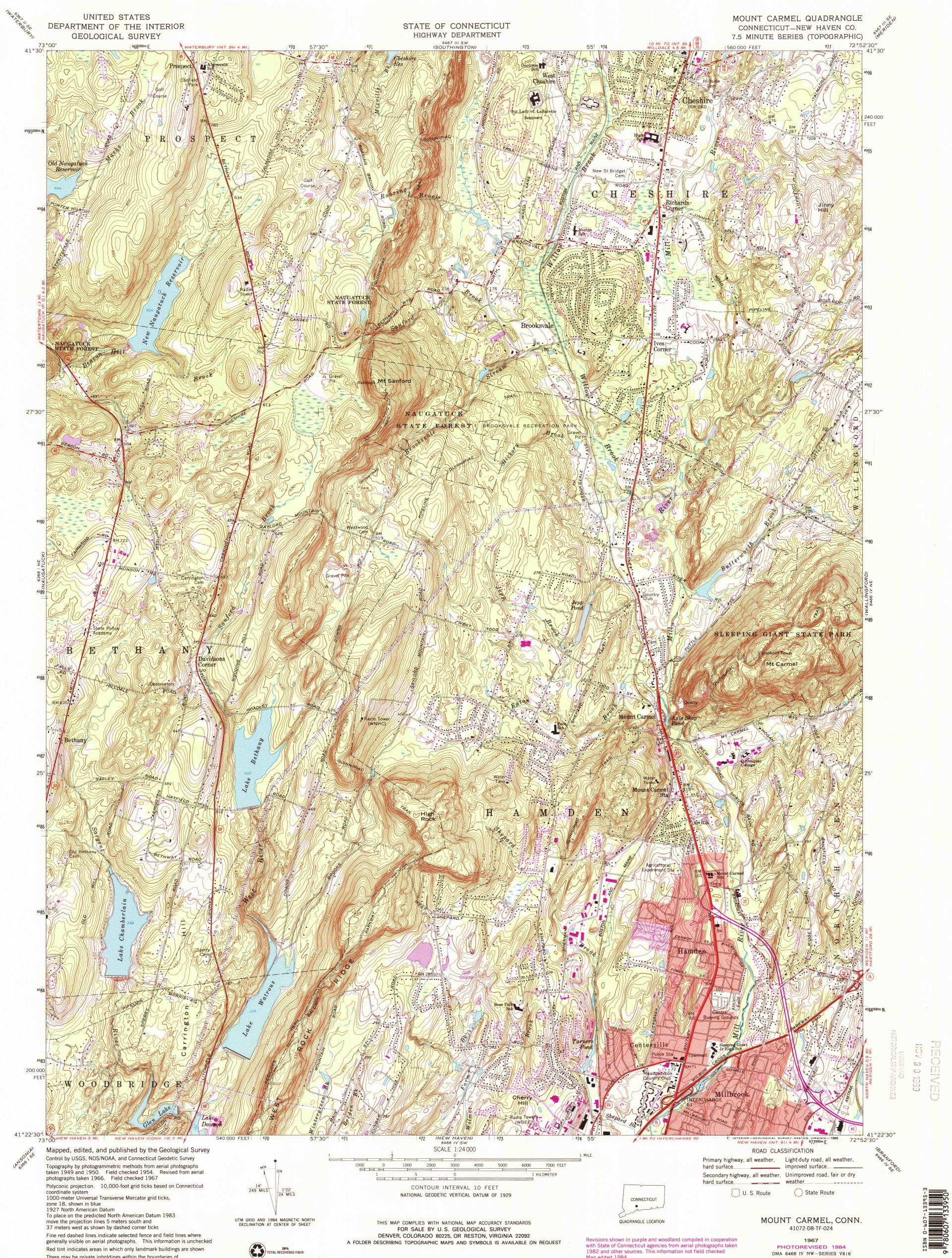
coordinate system 1000-meter Universal Transverse Mercator grid ticks, zone 18, shown in blue 1927 North American Datum To place on the predicted North American Datum 1983 move the projection lines 5 meters south and 37 meters west as shown by dashed corner ticks
