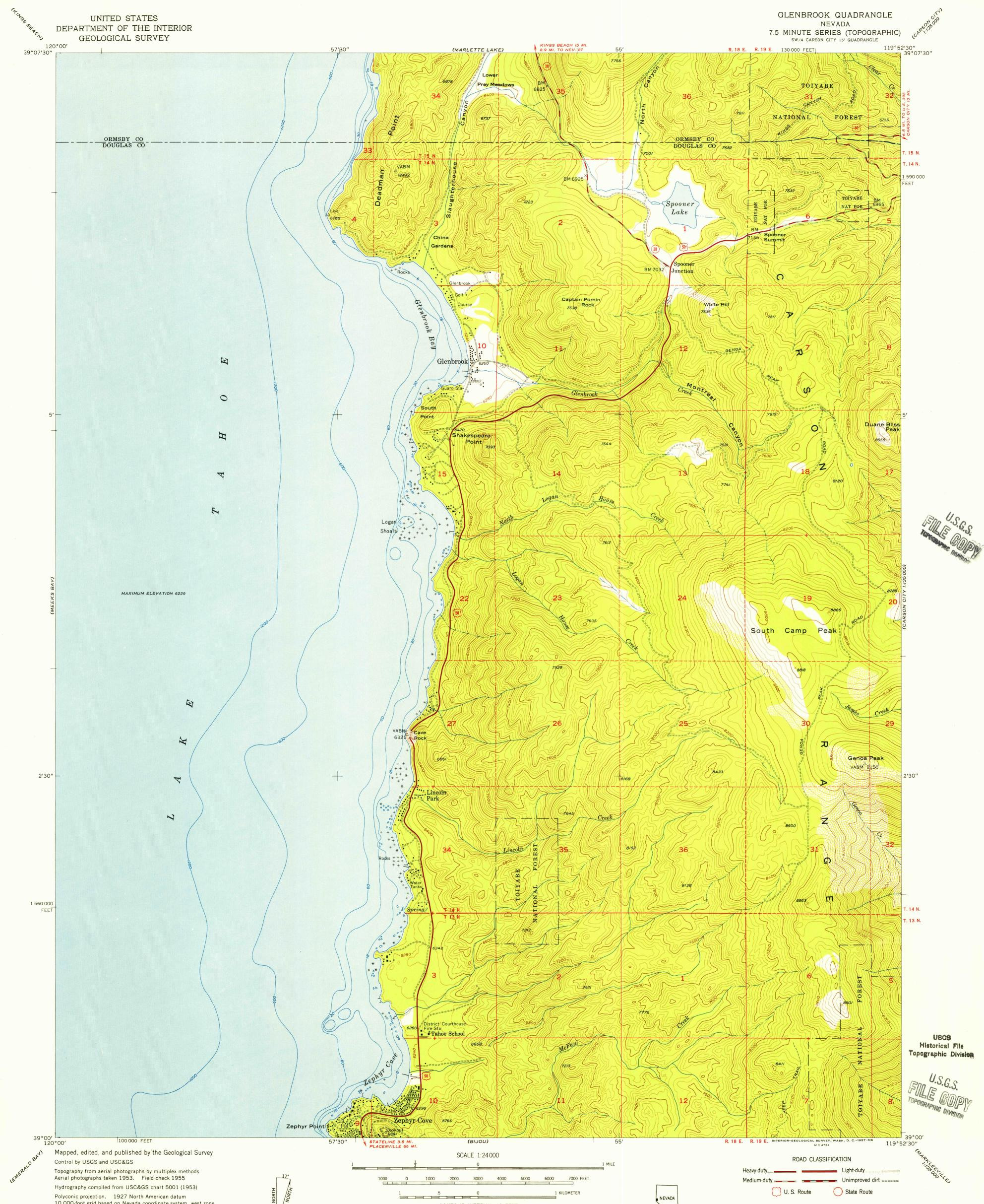
Polyconic projection. 1927 North American datum 10,000-foot grid based on Nevada coordinate system, west zone
