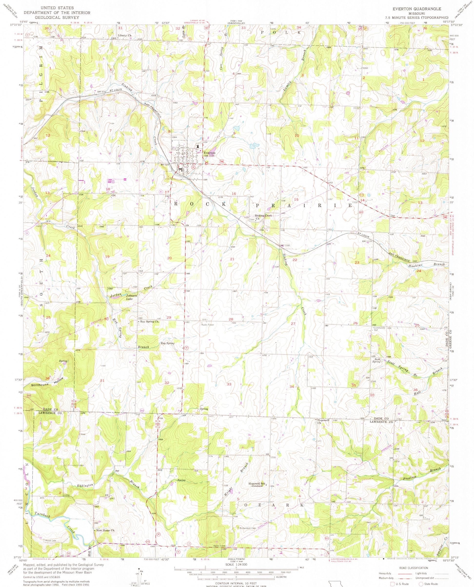
Aerial photographs taken 1950. Field check 1955-1956 Polyconic projection. 1927 North American datum 10,000-foot grid based on Missouri coordinate system, west zone 1000-metre Universal Transverse Mercator grid ticks, zone 15, shown in blue
