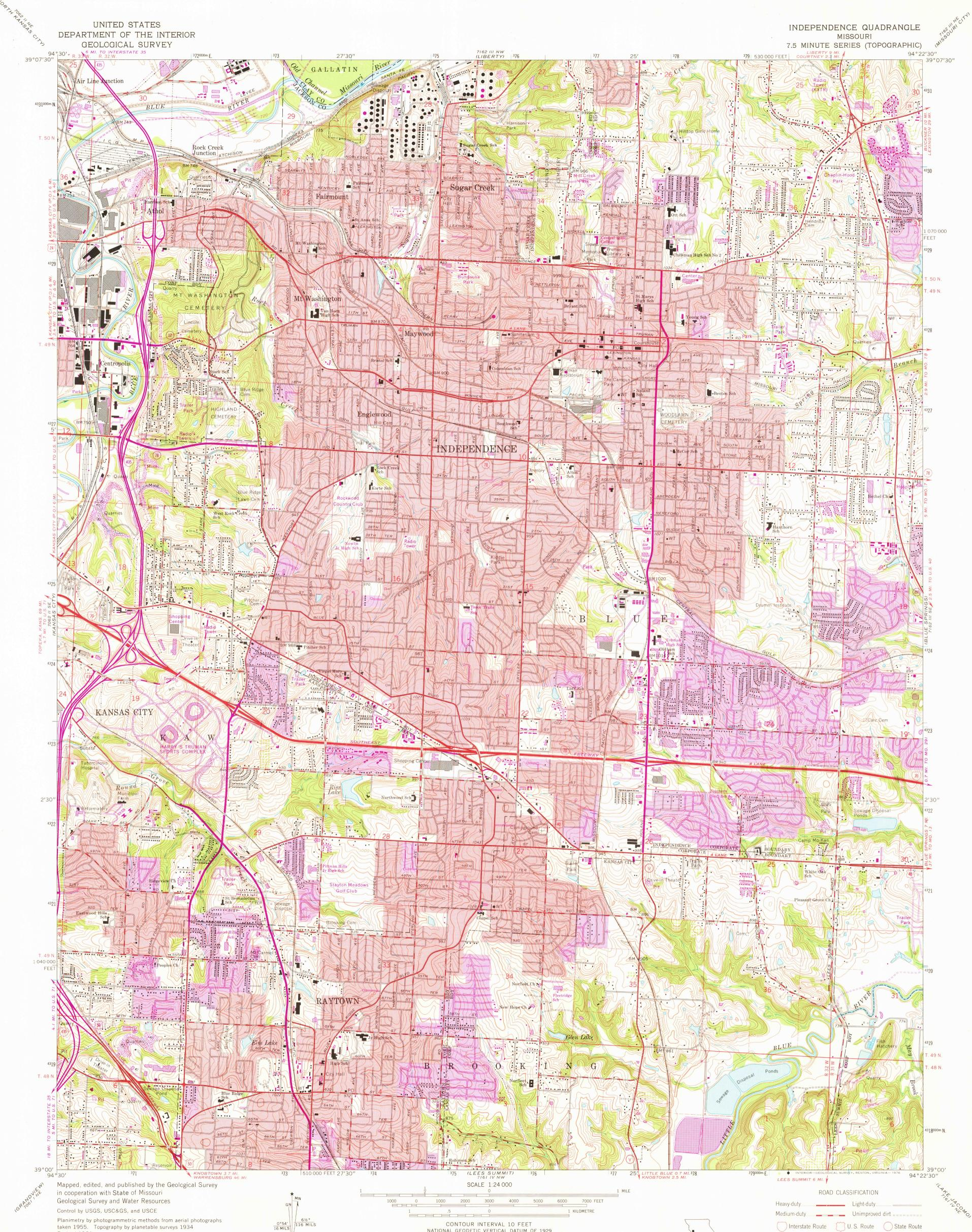
Planimetry by photogrammetric methods from aerial photographs taken 1955. Topography by planetable surveys 1934 Revised 1964
