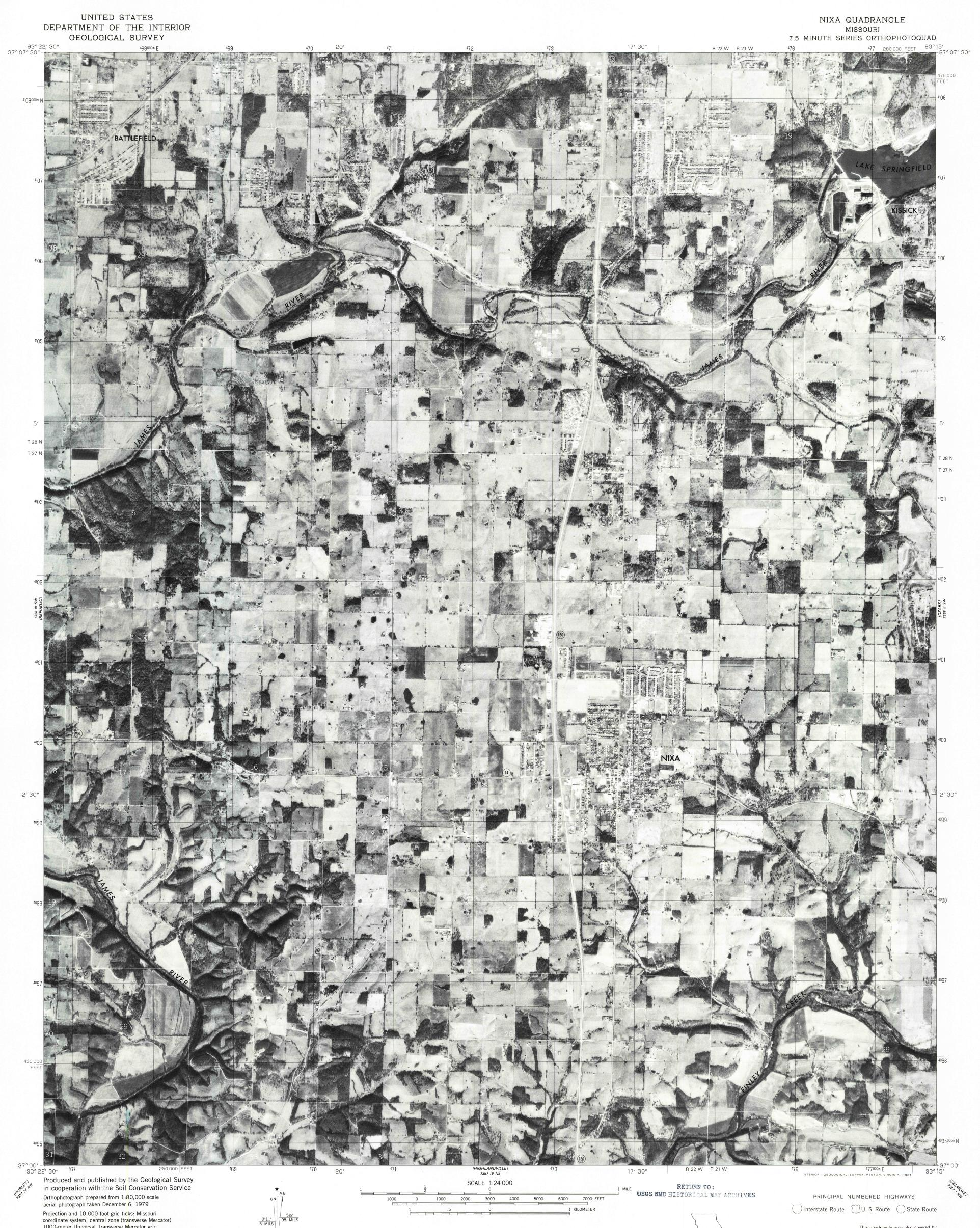
Projection and 10,000-foot grid ticks: Missouri coordinate system, central zone (transverse Mercator) 1000-meter Universal Transverse Mercator grid, zone 15. 1927 North American Datum To place on the predicted North American Datum 1983 move the projection lines 3 meters south and 16 meters east as shown by dashed corner ticks
