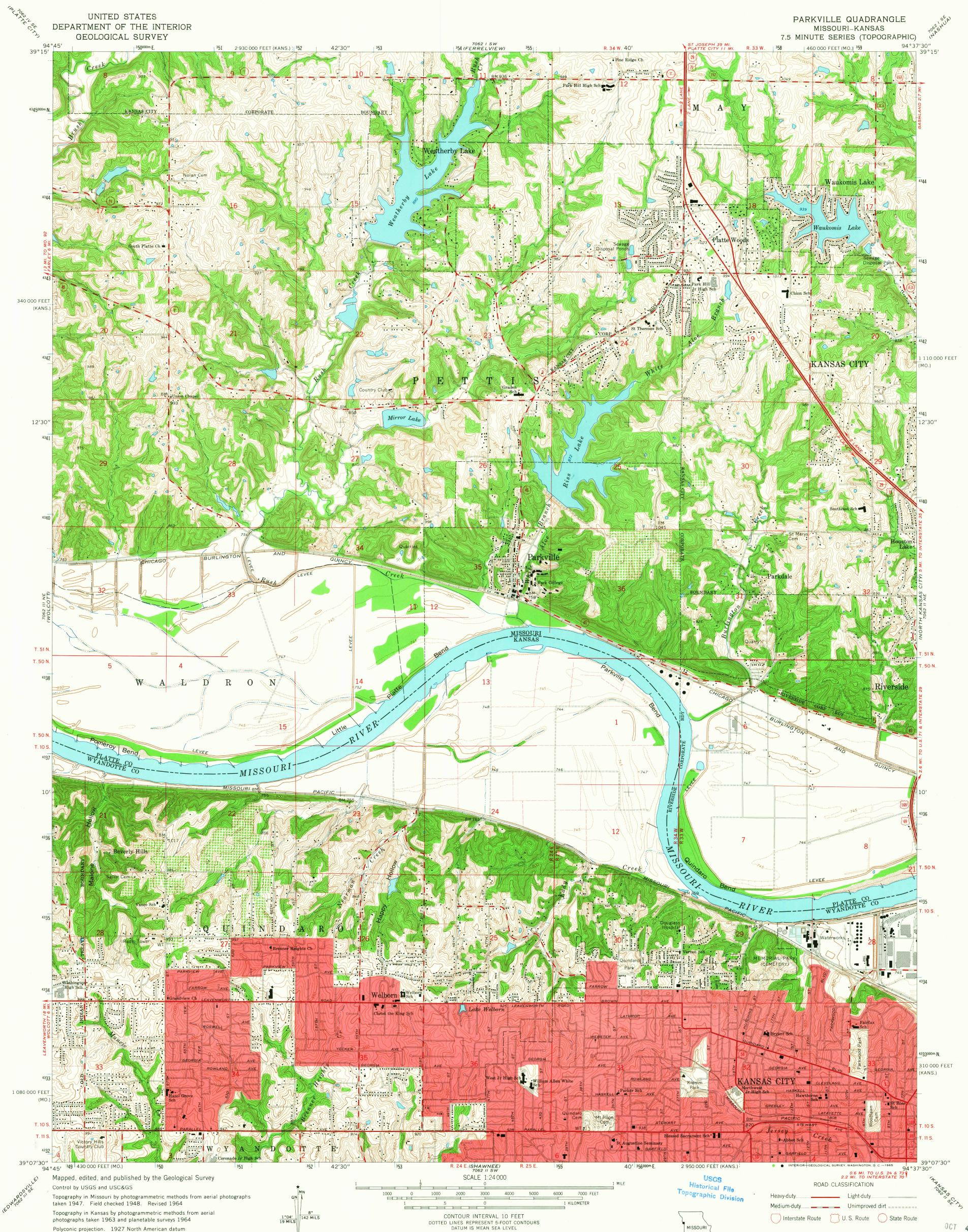
Polyconic projection. 1927 North American datum 10,000-foot grids based on Missouri coordinate system, west zone and Kansas coordinate system, north zone 1000-meter Universal Transverse Mercator grid ticks, zone 15, shown in blue
