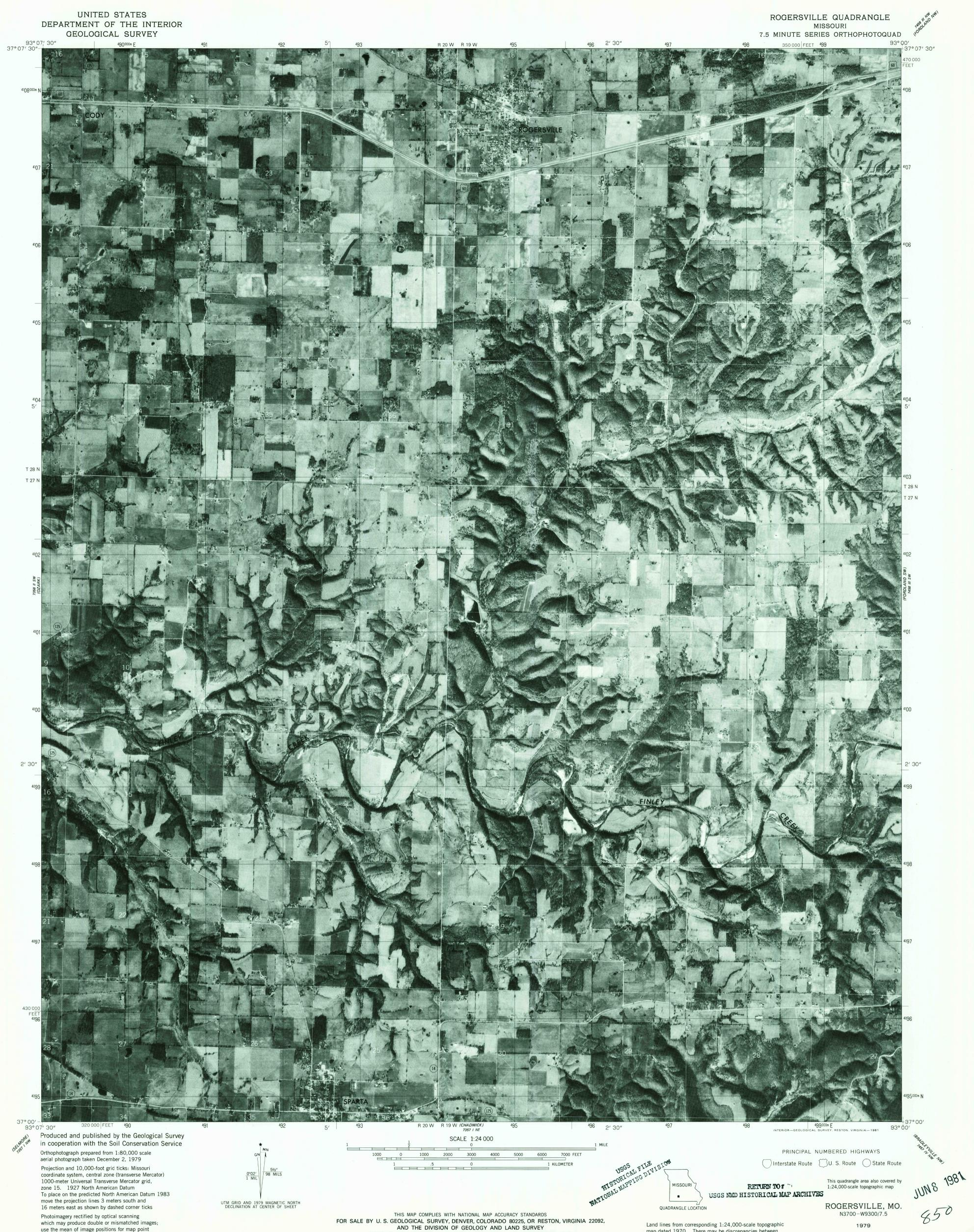
coordinate system, central zone (transverse Mercator) 1000-meter Universal Transverse Mercator grid, zone 15. 1927 North American Datum To place on the predicted North American Datum 1983 move the projection lines 3 meters south and 16 meters east as shown by dashed corner ticks
