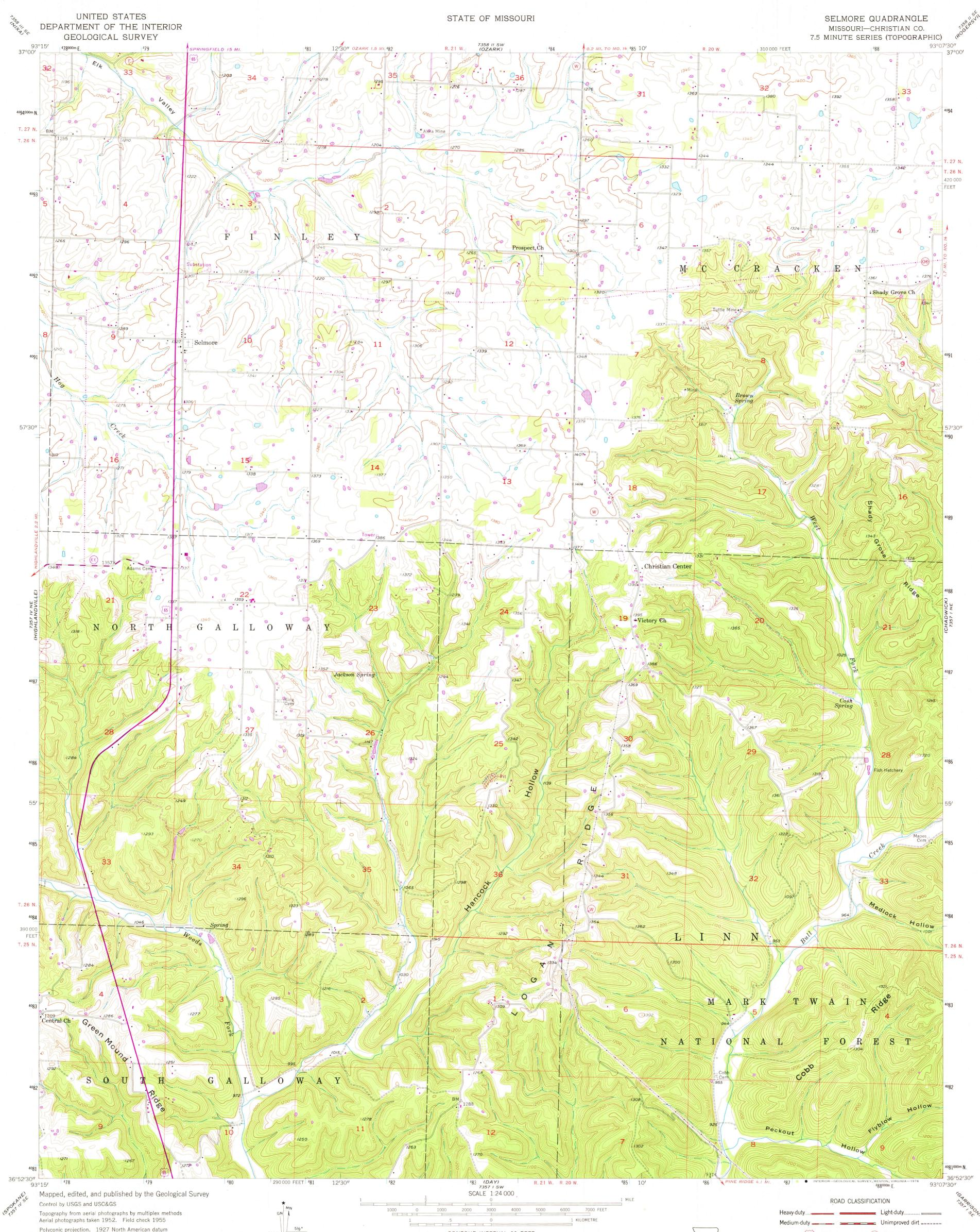
Polyconic projection. 1927 North American datum 10,000-foot grid based on Missouri coordinate system, central zone 1000-metre Universal Transverse Mercator grid ticks, zone 15, shown in blue
