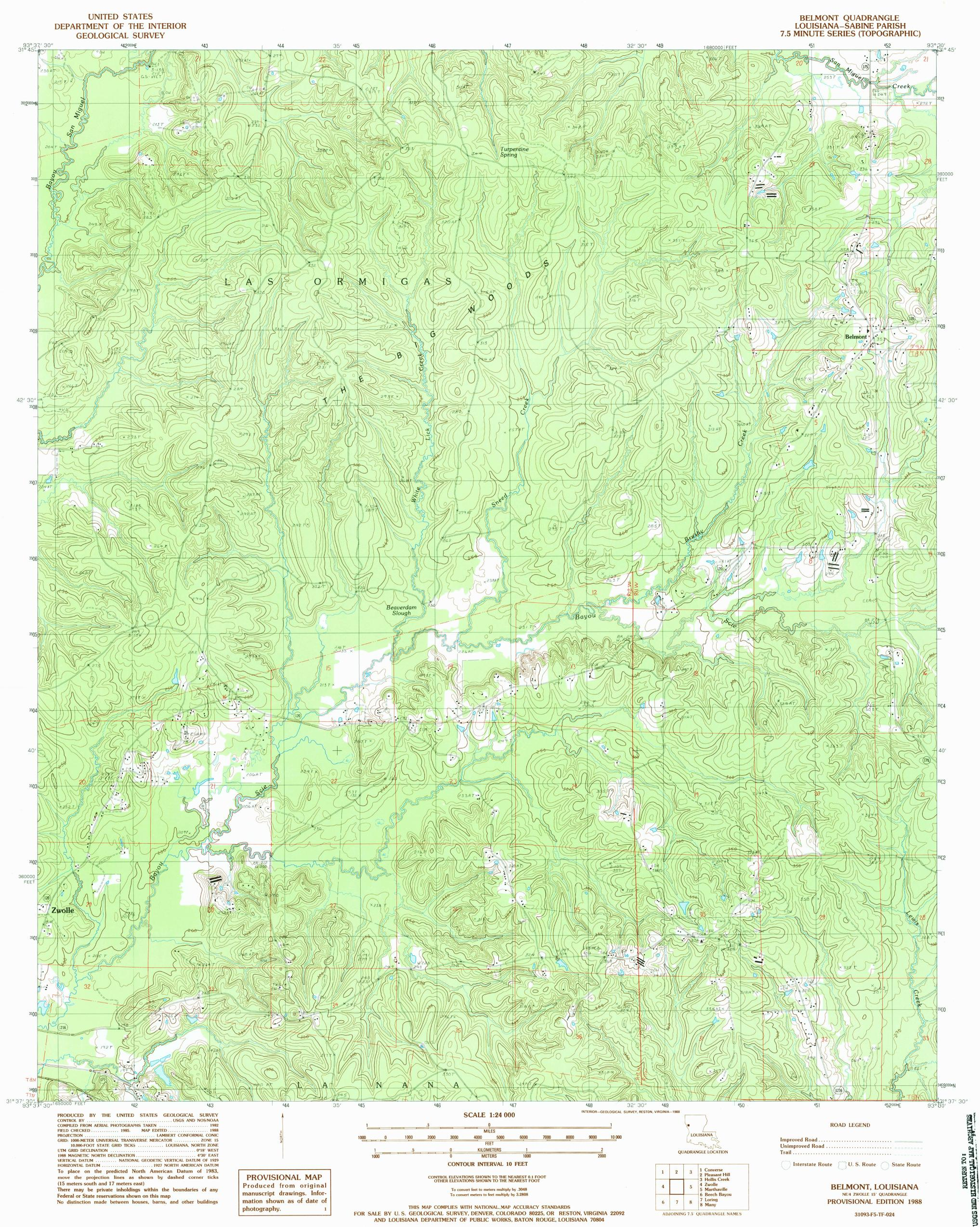
.... NATIONAL GEODETIC VERTICAL DATUM OF 1929 VERTICAL DATUM ... HORIZONTAL DATUM ... ..... 1927 NORTH AMERICAN DATUM To place on the predicted North American Datum of 1983, move the projection lines as shown by dashed corner ticks (15 meters south and 17 meters east) There may be private inholdings within the boundaries of any Federal or State reservations shown on this map No distinction made between houses, barns, and other buildings
