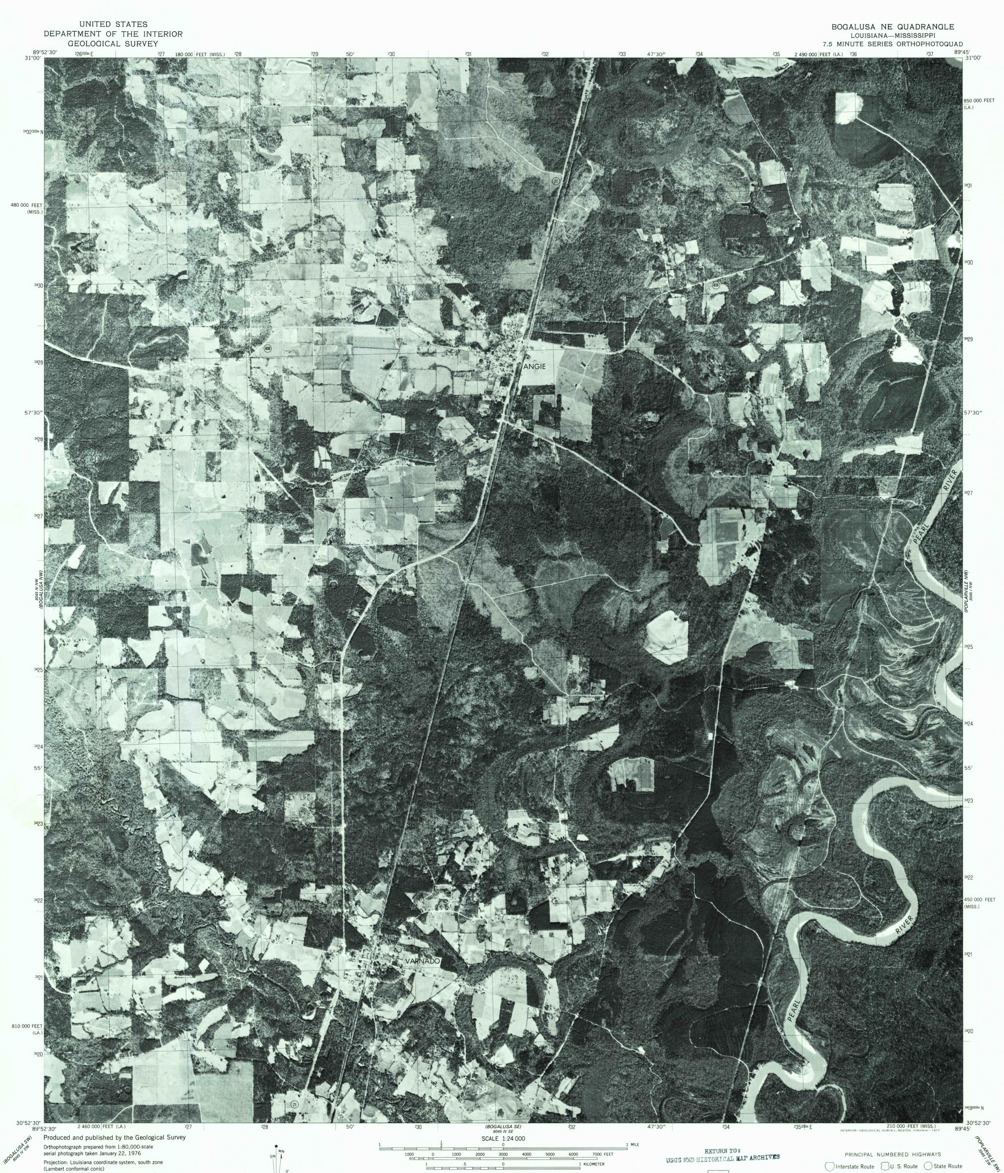
(Lambert conformal conic) 10,000-foot grid ticks based on Louisiana coordinate system, south zone and Mississippi coordinate system east zone 1000-meter Universal Transverse Mercator grid, zone 16. 1927 North American datum
