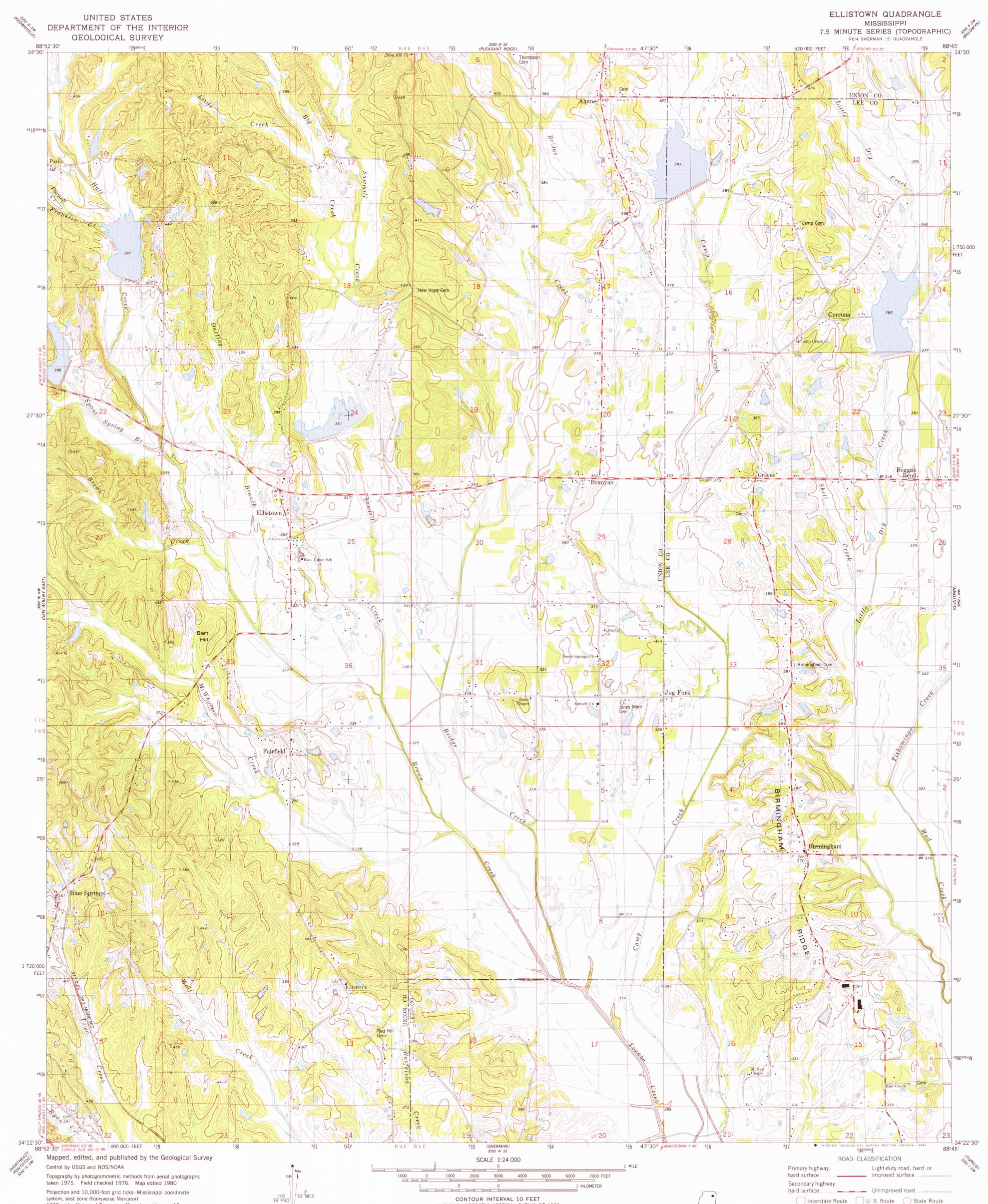
system, east zone (transverse Mercator) 1000-meter Universal Transverse Mercator grid, zone 16 1927 North American Datum To place on the predicted North American Datum 1983 move the projection lines 9 meters south and 5 meters east as shown by dashed corner ticks
