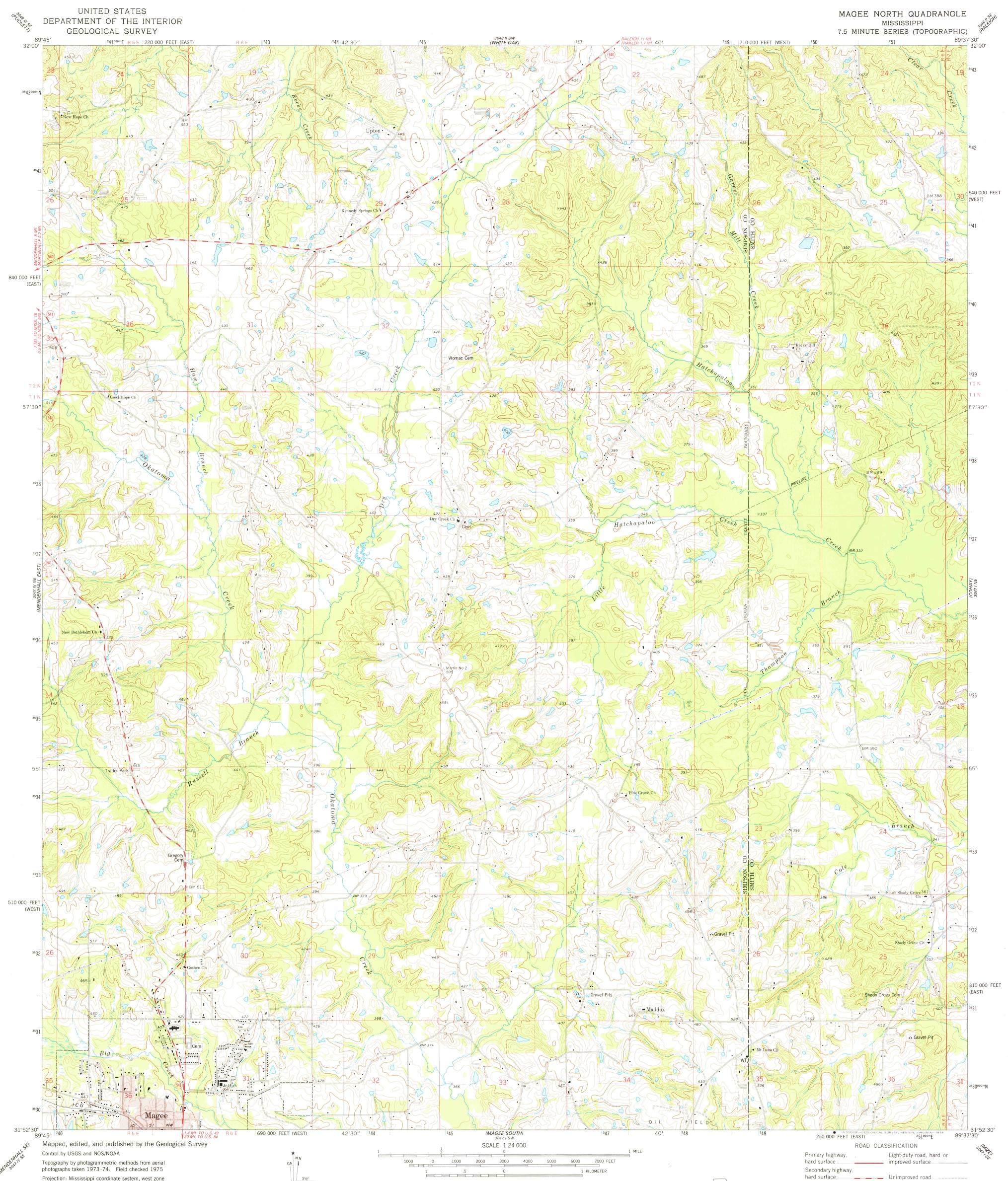
(transverse Mercator) 10,000-foot grid ticks based on Mississippi coordinate system, west and east zones 1000-meter Universal Transverse Mercator grid ticks, zone 16, shown in blue. 1927 North American datum Red tint indicates area in which only landmark buildings are shown Fine red dashed lines indicate selected fence and field lines where
